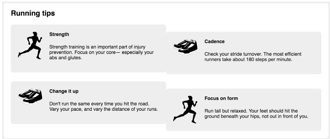
Figure 4.18 Removing position-related properties from the media object allows the grid system to position and size them accordingly.
