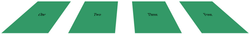
Figure 15.16 Make the elements share a common perspective by using the perspective property on a common ancestor element.
