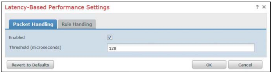
Figure 11-23 Latency-Based Packet Thresholding
