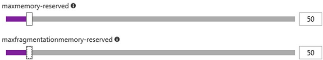
Figure 3-21. This is how we configure the reserved memory of our Redis instance. This section is available under the Advanced Settings page of the Redis instance blade on the Azure Portal
