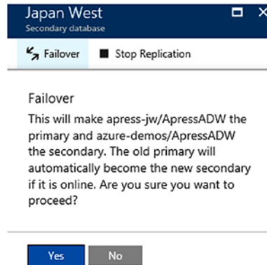
Figure 1-14. A Failover action on the Japan West replica. Azure will manage the promotion and the demotion of the respective primary/secondary DBs.
