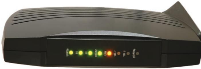
**Figure 6-1.** *Cable modem*
