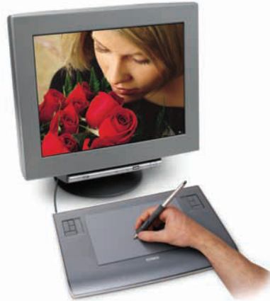
Figure 3-17: This Wacom pen and tablet set is easier to draw with than a mouse and enables you to easily vary the brush width as you draw.
