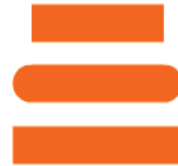
Figure 3-4: These lines were all drawn 88 pixels long, but the bottom two lines have caps, so they're longer.
