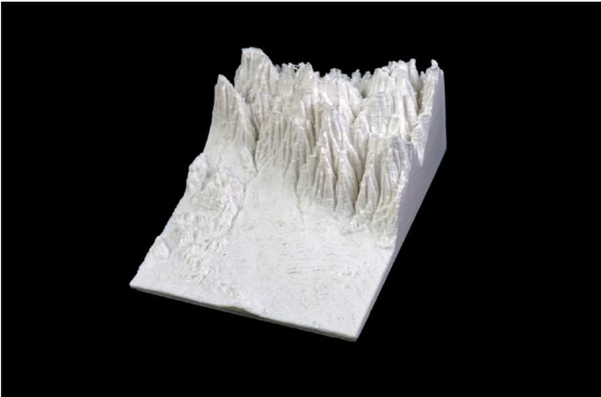
**Figure 10-1.** Pasadena terrain model created by Terrain2STL, high vertical exaggertion, printed flat (as shown)
