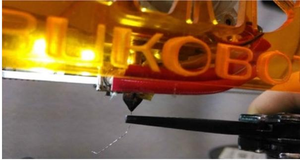
**Figure 5-8.** *Using the wire brush bristle to clear out the nozzle*
