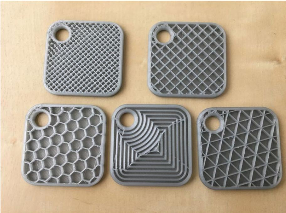
**Figure 3-9.** *Typical infill patterns*
