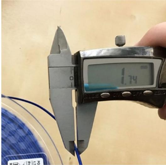
**Figure 2-11.** *Checking filament diameter with a pair of calipers*
