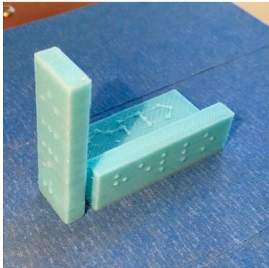
*Figure 12-4. 3D printed Braille in three orientations*
