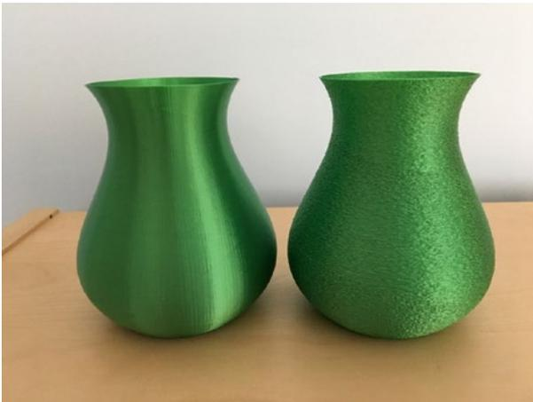
**Figure 8-2.** Two spiralized vases, the one on the right with “fuzzy skin”
