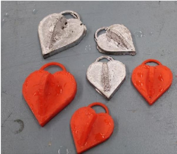
**Figure 8-11.** *Heart patterns and finished aluminum cast pieces*
