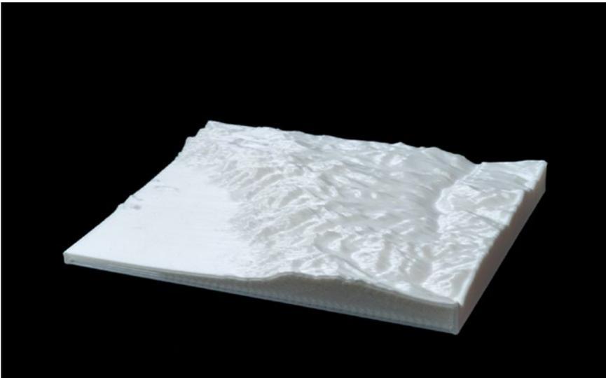
**Figure 10-2.** Mt. Whitney area, no vertical exaggeration, printed vertically
