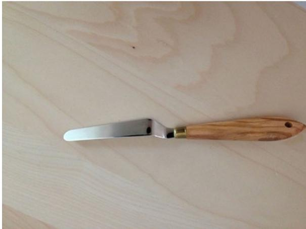
**Figure 5-3.** *A painting knife is a good tool to remove a part from a tape-covered platform*
