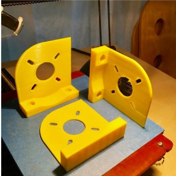
**Figure 9-7.** Motor mount printed in three orientations
