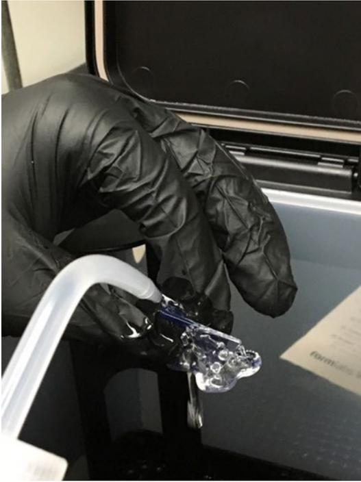
**Figure 5-10.** *A resin print being washed with alcohol in a Formlabs wash station*
