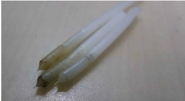
**Figure 5-6.** *Nylon with residue of overheated plastic*
