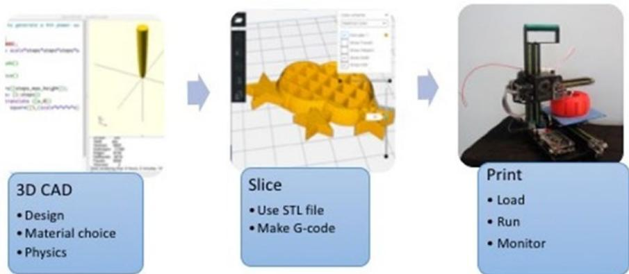
*Figure 3-1. 3D-printing workflow*
