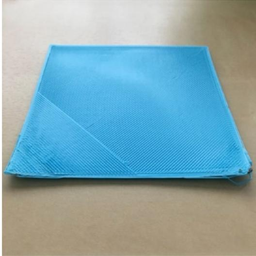
*Figure 2-13. An ABS part that pulled up from the heated bed*
