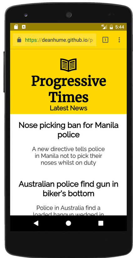
Figure 5.1 The theme_color property in the web app manifest can be used to style your web app.
