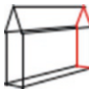
Figure 4-8. Perspective image with R_y=-60 , zfp=-100 , xc=40 , yc=70 , xfp=100 , zfp=-80
