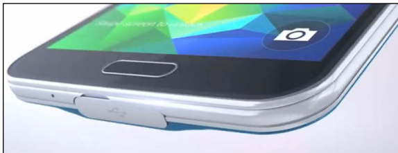
Figure 2-5: The multi-purpose jack on your phone.
