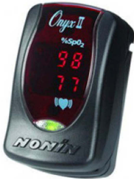
Figure 16-10: A Onyx II wireless pulse oximeter from Nonin.
