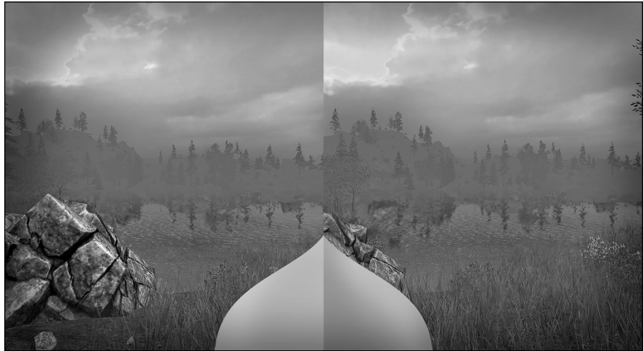
FIGURE 2-13: Using a virtual nose to prevent simulator sickness.
