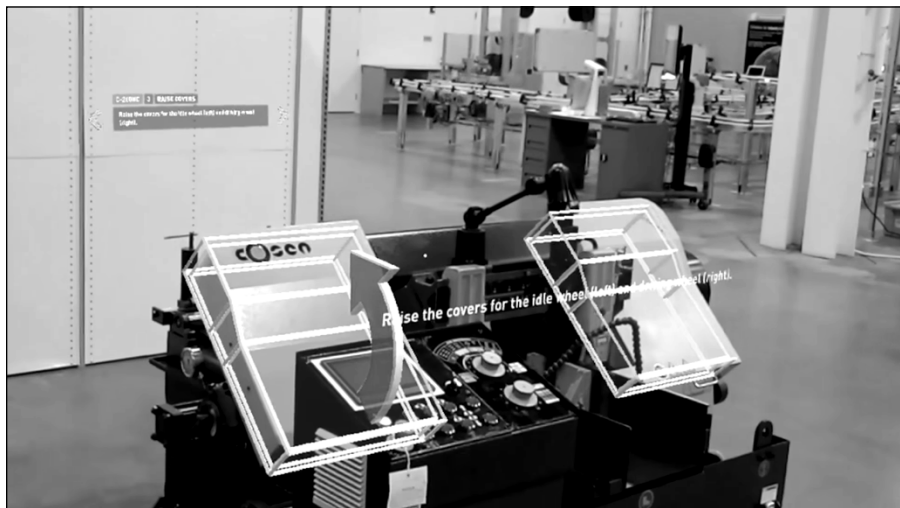
FIGURE 11-6: Scope AR's WorkLink application in use.
