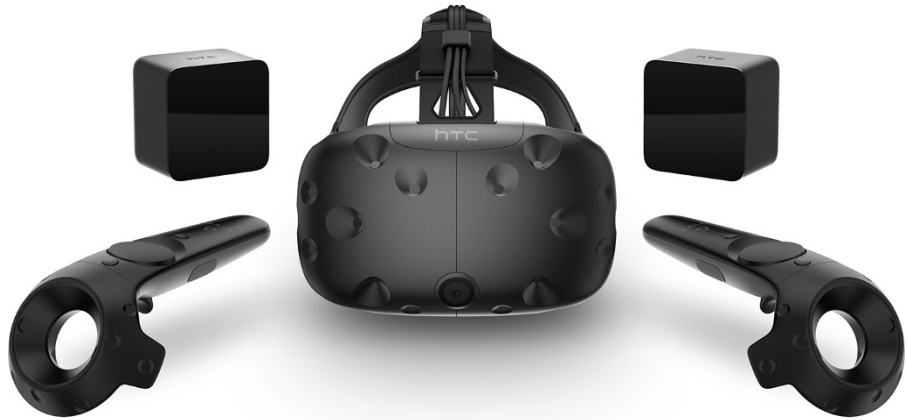
FIGURE 4-1: HTC Vive, controllers, and sensors.
