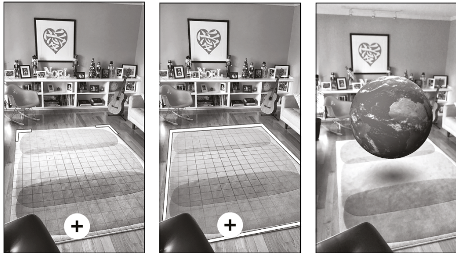
FIGURE 3-5: Placing virtual objects via touch in mobile AR.
