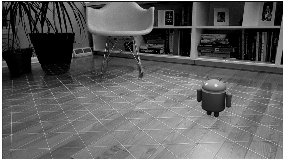
FIGURE 3-6: An example of an ARCore grid following the user's gaze.
