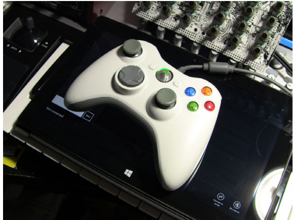
Figure 21.10 The Xbox controller for Windows sitting on my Surface with Windows RT. Yes, the Xbox controller works on Windows RT. You can tell I've had it forever because it's a white one. There are a number of controllers you can use, as long as XInput recognizes them without an additional driver install.
