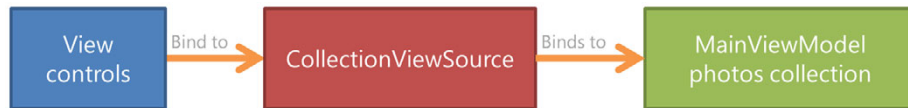
Figure 10.4 The relationship between the ListView and GridView controls, the CollectionViewSource , and the viewmodel
