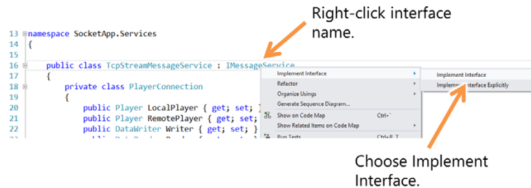
Figure 20.4 Implement the interface to pull in the missing event and method declarations.
