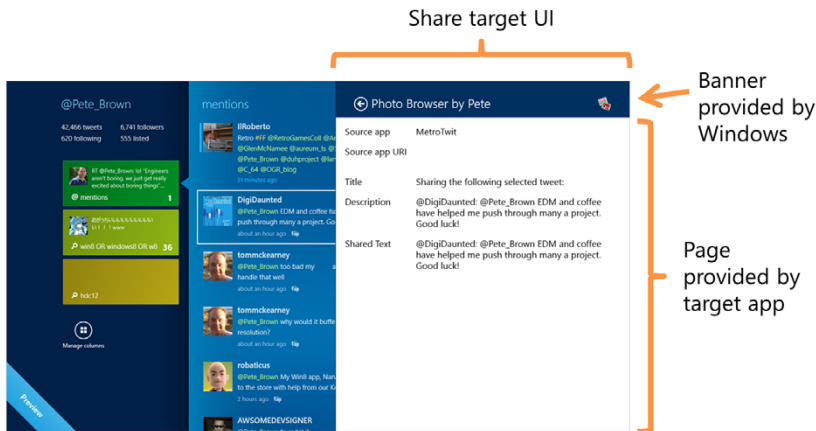
Figure 14.7 The PhotoBrowser app's Share Target UI shown with MetroTwt as the share source. Windows built and animated the flyout as well as its header.
