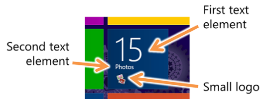
Figure 12.11 A simple text notification using the TileSquareBlock template with two text elements showing actual data from the app. Notice the small logo. Given its 30 x 30 size, a version without rotated images would work better here.
