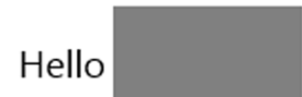
Figure 6.3 Two elements in a white canvas. Note how the rectangle obscures the “World!” part of the “Hello World!” TextBlock text.
