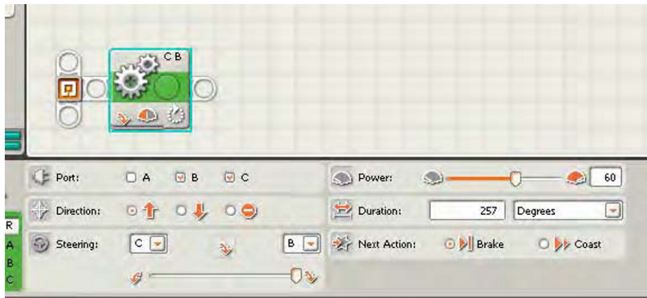
Figure 4-4. A Move block being set to pivot the DemoBot 180 degrees by using the value of 257.4 as the Duration and the steering set to the far right.
