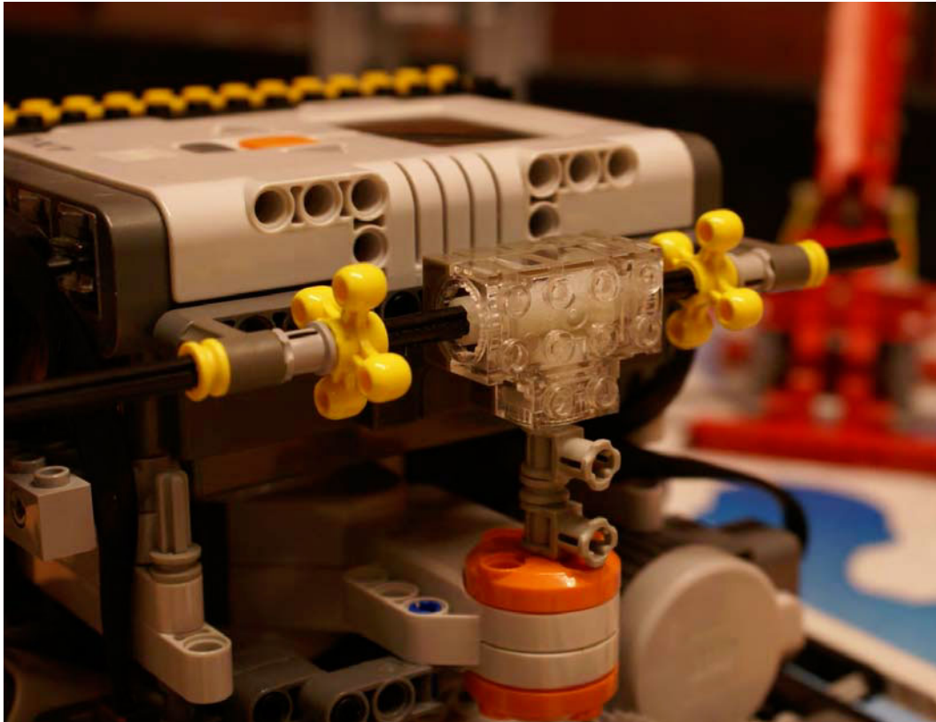
Figure 9-3. A middle-mounted NXT motor connected to a bevel gear box to change the direction of the motor's output
