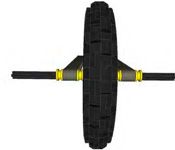
Figure 3–4. With the axle and wheel supported evenly on both ends, the friction is reduced drastically, and you get a much stabler drive system for the robot.
