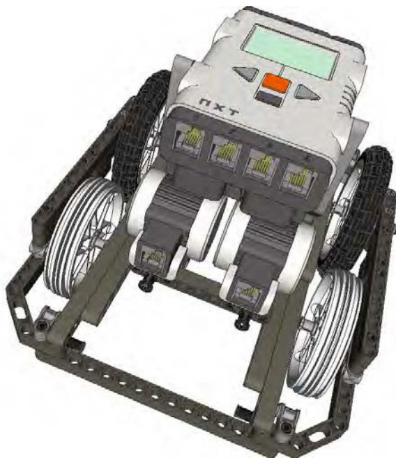
Figure 6-1. DemoBot has a flat rear surface on the chassis to allow for flush contact with the wall when squaring up.
