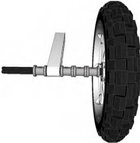
Figure 2-18. Multiple bushing spacing on a wheel axle, moving the wheel further from the chassis causing more friction
