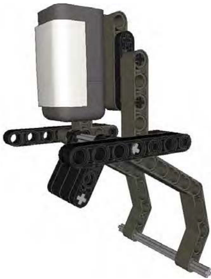
Figure 7-12. With the bumper pushed the black beams are removed from the view of the Light sensor.
