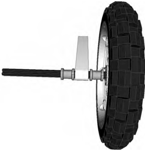
Figure 2-17. Single bushing spacing on wheel axle
