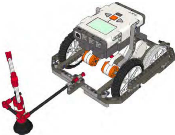
Figure 8–5. Once the hook is behind the object, the robot simply moves backwards to retrieve the item to base.
