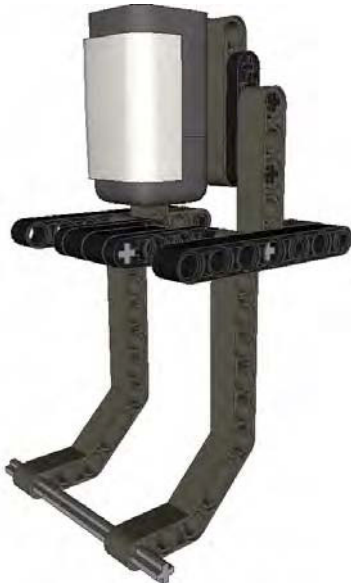
Figure 7-11. A Light Sensor being used to detect touch by a bumper that blocks the Light Sensor's path with black beams
