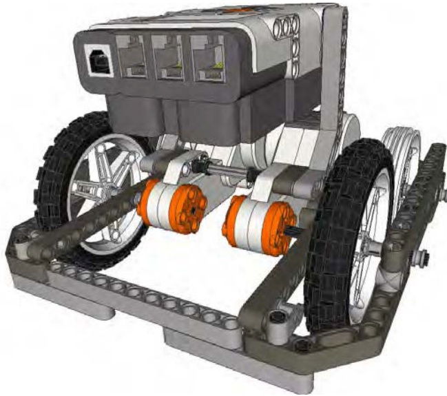
Figure 4–1. DemoBot is an example of a differential steering robot chassis design. The two motors are used to control the speed as well as the direction.
