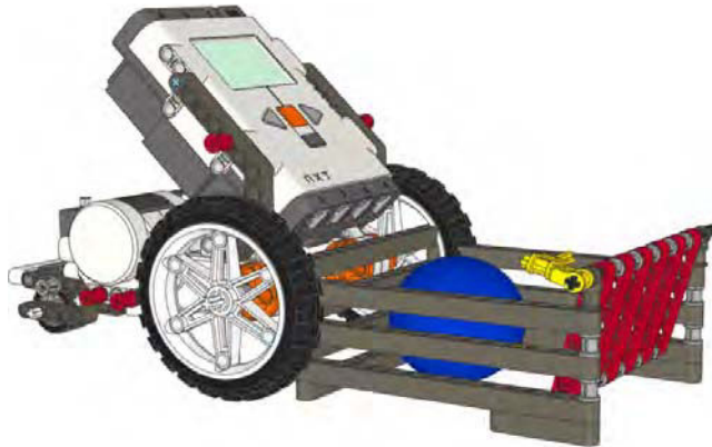
Figure 8-15. Once the ball enters the attachment, the door swings closed behind it, locking it inside.
