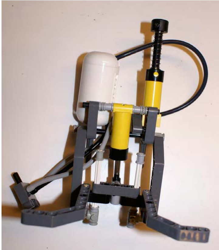
Figure 10–11. A robot's lifting attachment using pneumatics
