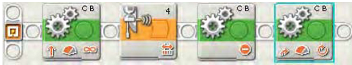
Figure 7-15. NXT-G code using an Ultrasonic Sensor for collision detection
