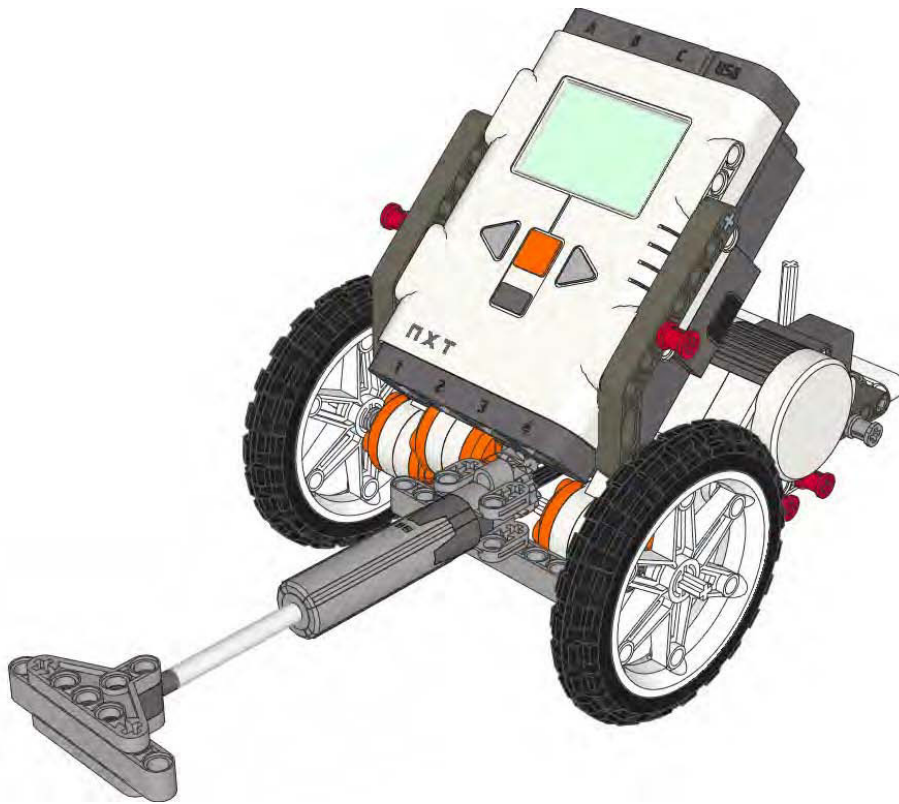
Figure 9–13. LEGO Power Functions actuator mounted to a robot as a pushing power attachment.
