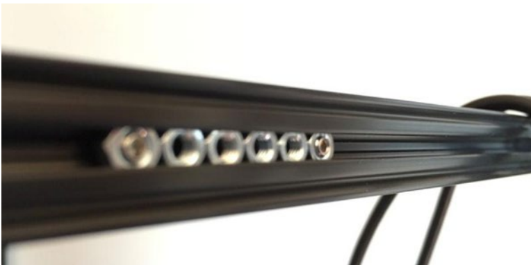
Figure 4-9. Adding extra nuts to frame members
