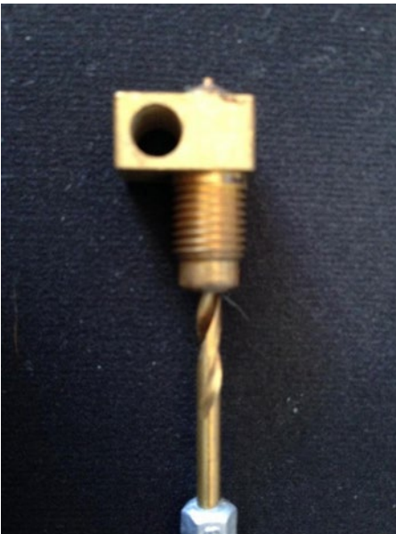
Figure 7-12. Proper size and location of drill bit for removing plastic
