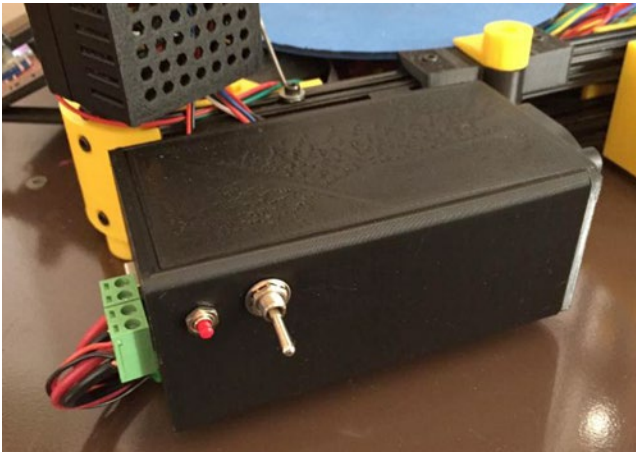
Figure 8-14. Electronics enclosure for Mini Kossel
