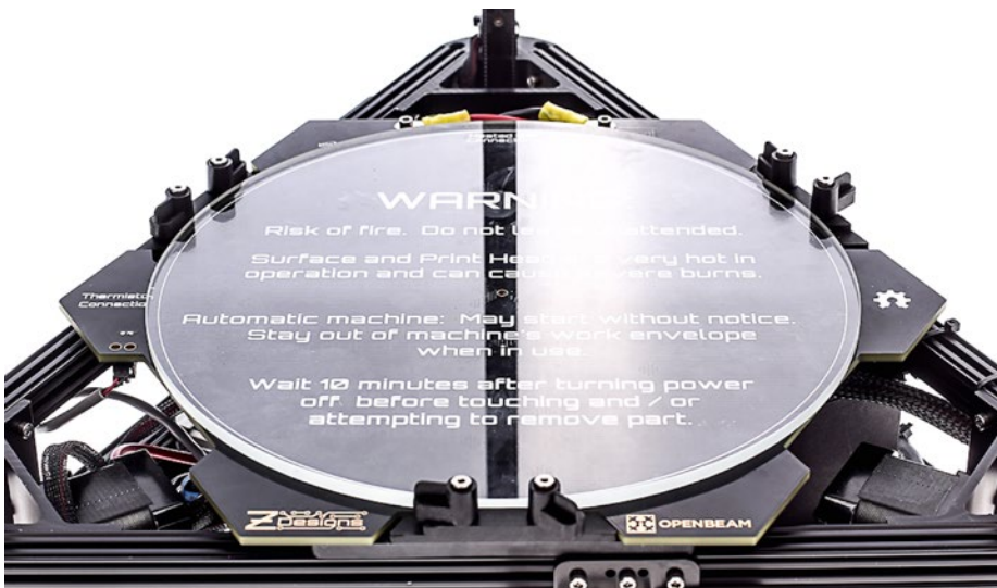
Figure 2-17. Heated build platform (image courtesy of Seattle Automationz, LLC)
