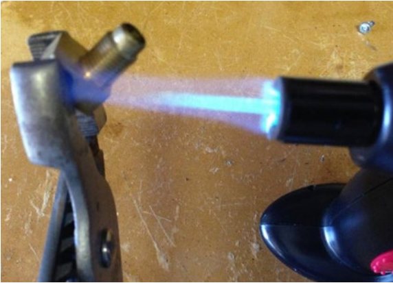
Figure 7-11. Place the nozzle in the flame
