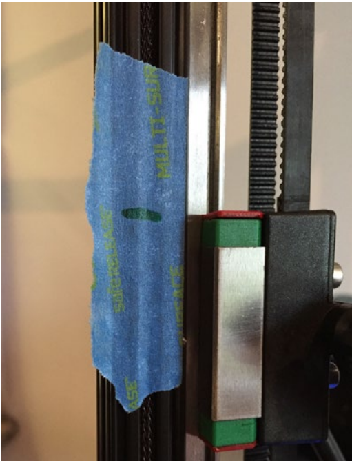
Figure 2-4. Marking the carriage position
