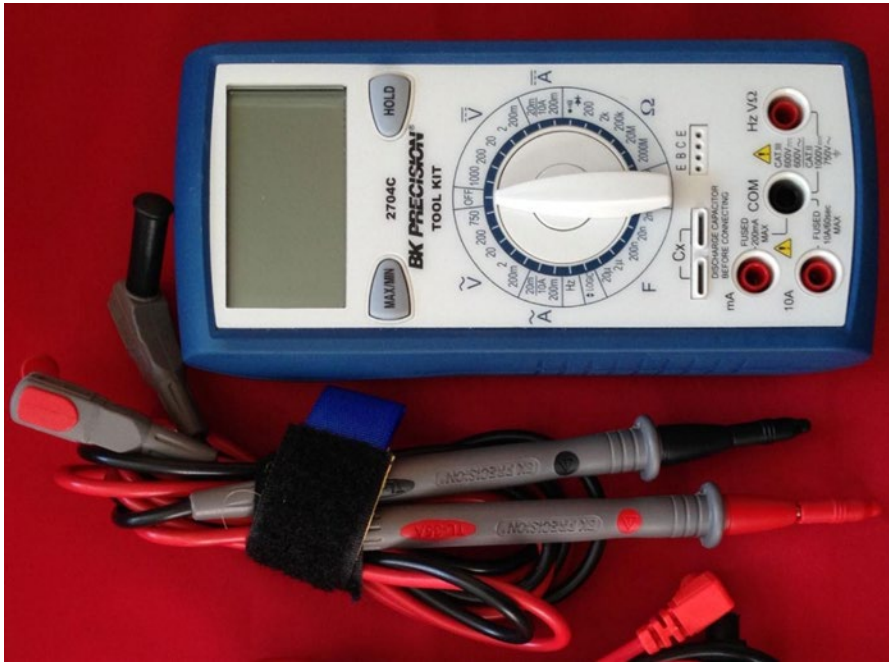
Figure 4-4. Advanced digital multimeter
