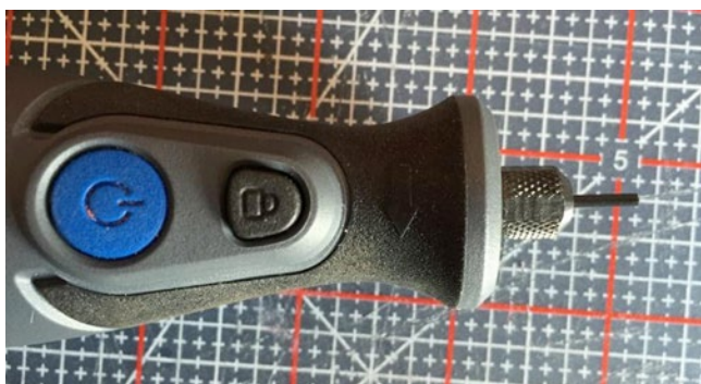
Figure 6-15. Preparing Dremel for plastic welding
