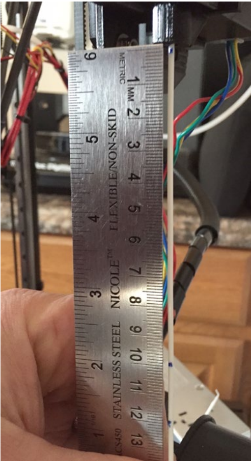
Figure 5-23. Marking filament at 0, 100, and 120mm
