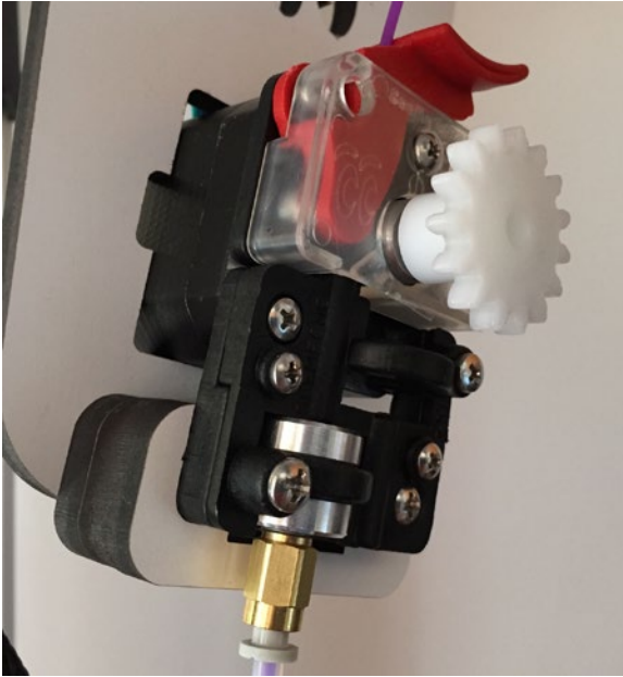
Figure 2-6. Extruder assembly (EZStruder by SeeMeCNC)
