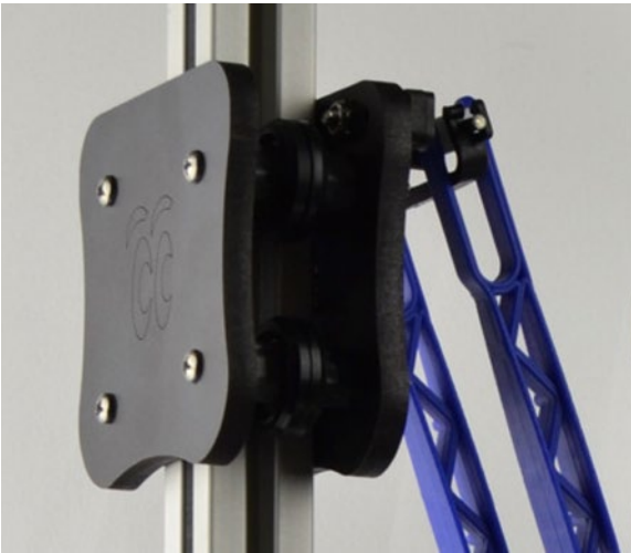
Figure 2-13. Roller carriage (courtesy of SeeMeCNC)
