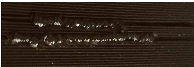
Figure 6-16. Plastic welding example
