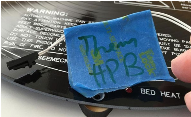
Figure 4-13. Ad hoc wire labels
