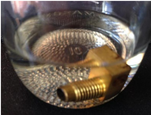
Figure 7-14. Soaking the nozzle in acetone (ABS only)
