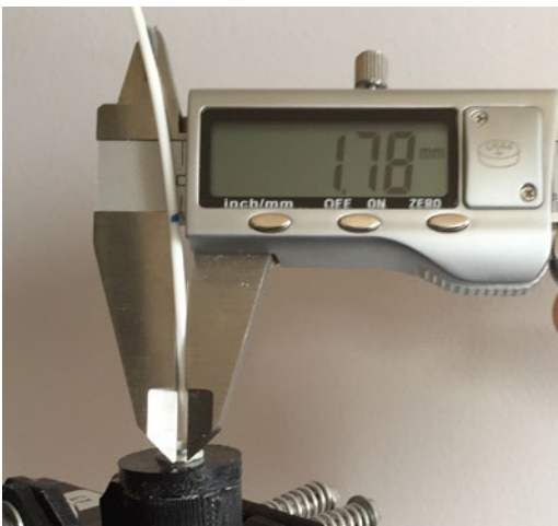
Figure 5-26. Measuring filament diameter
