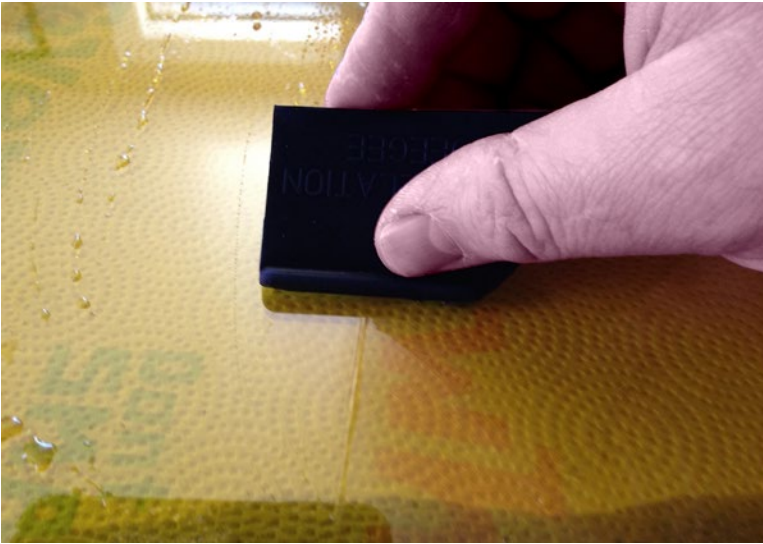
Figure 1-13. Go over the seam(s)
