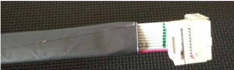
Figure 4-11. After wrapping the LCD cables
