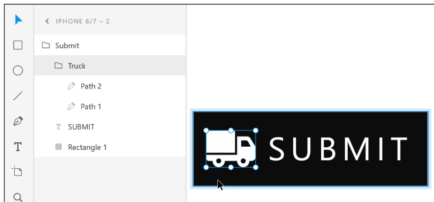
FIGURE 4-7: In this example, there is a group named Truck inside another group named Submit.
