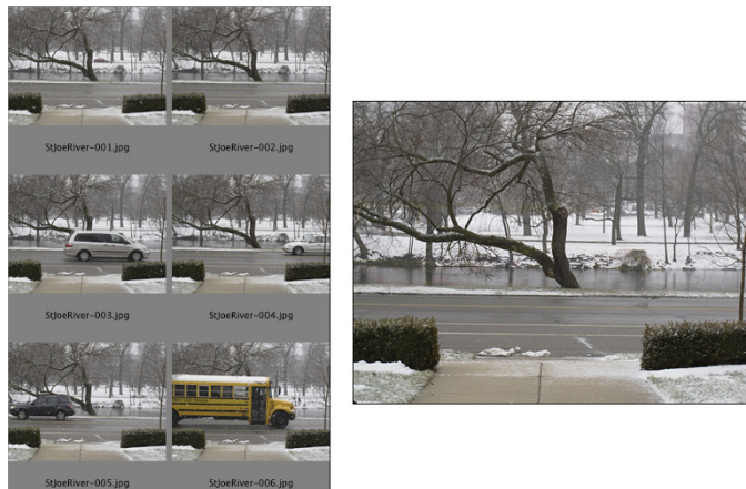
FIGURE 18-3: The cars on either side of the river, the bus, and even the falling snow are removed using Median.
