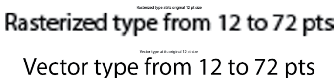
FIGURE 11-3: Using text as an example shows the advantage of vector artwork when scaling.
