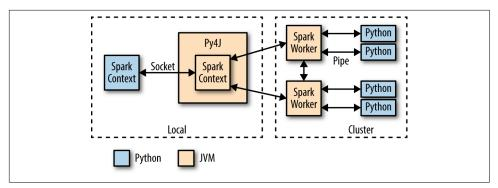
Figure 11-1. PySpark internal architecture
