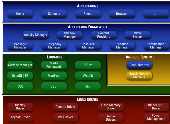
Figure 2-3: How the Android application framework stacks up.
