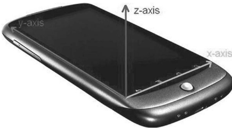
Figure 3-20. The accelerometer axes on an Android phone. The z axis points out of the phone
