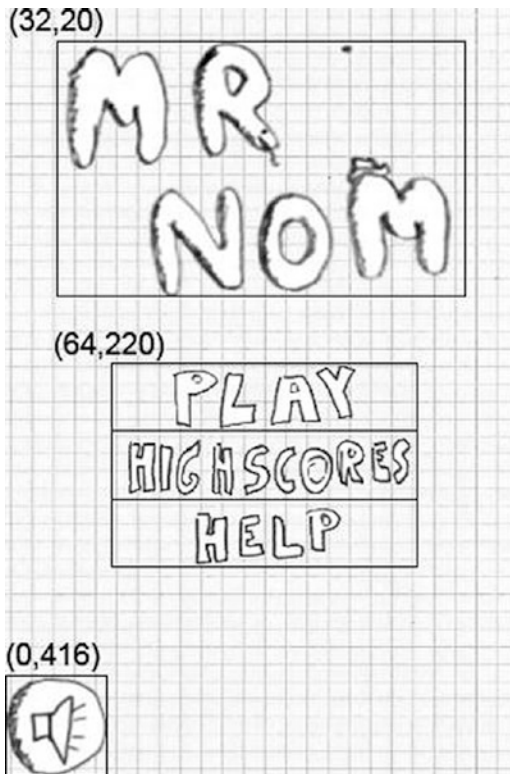
Figure 6-2. The main menu screen. The coordinates specify where we'll render the different images, and the outlines show the touch areas.
