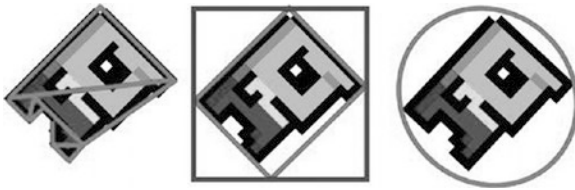
Figure 8-9. Rotated bounding shapes, with the center of the object as the rotation point
