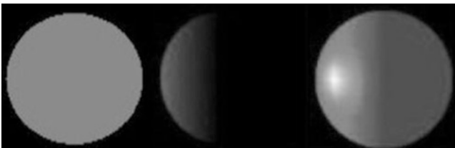
Figure 11-3. Different material/light types. Left: ambient only. Center: Diffuse only. Right: Ambient and diffuse with specular highlight
