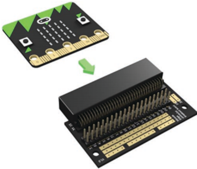
Figure 4-4. Inserting micro:bit into the edge connector breakout board (image courtesy of Kitronik: https://www.kitronik.co.uk/ )
