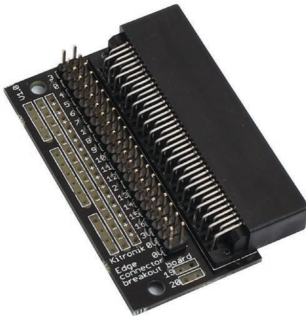
Figure 1-4. Kitronik edge connector breakout board (image courtesy of Kitronik: https://www.kitronik.co.uk/5601b-edge-connector-breakout-board-for-bbc-microbit-pre-built.html )
