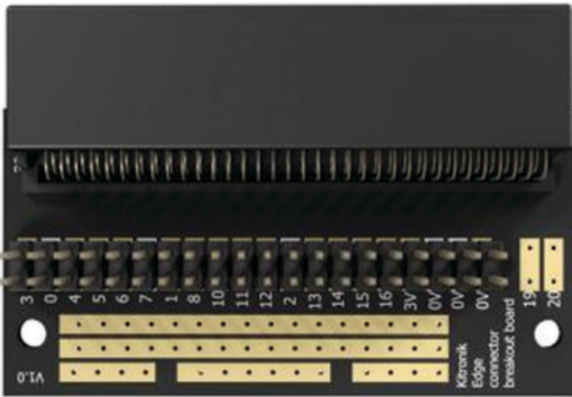
Figure 4-3. Major areas of the edge connector breakout board (image courtesy of Kitronik: https://www.kitronik.co.uk/ )
