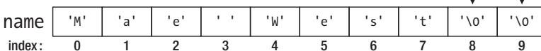
Figure 5-5. An array of elements of type char initialized with a string literal
