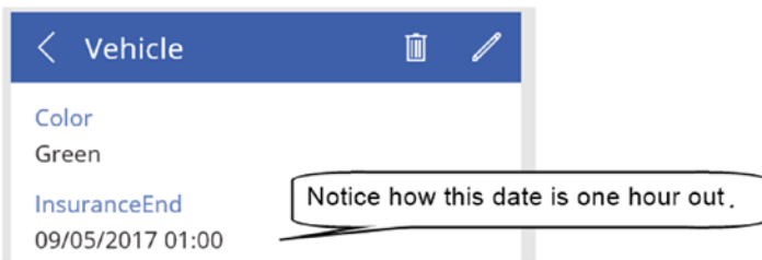
Figure 8-18. The date that PowerApps retrieves is incorrect when we set the TimeZone to UTC
