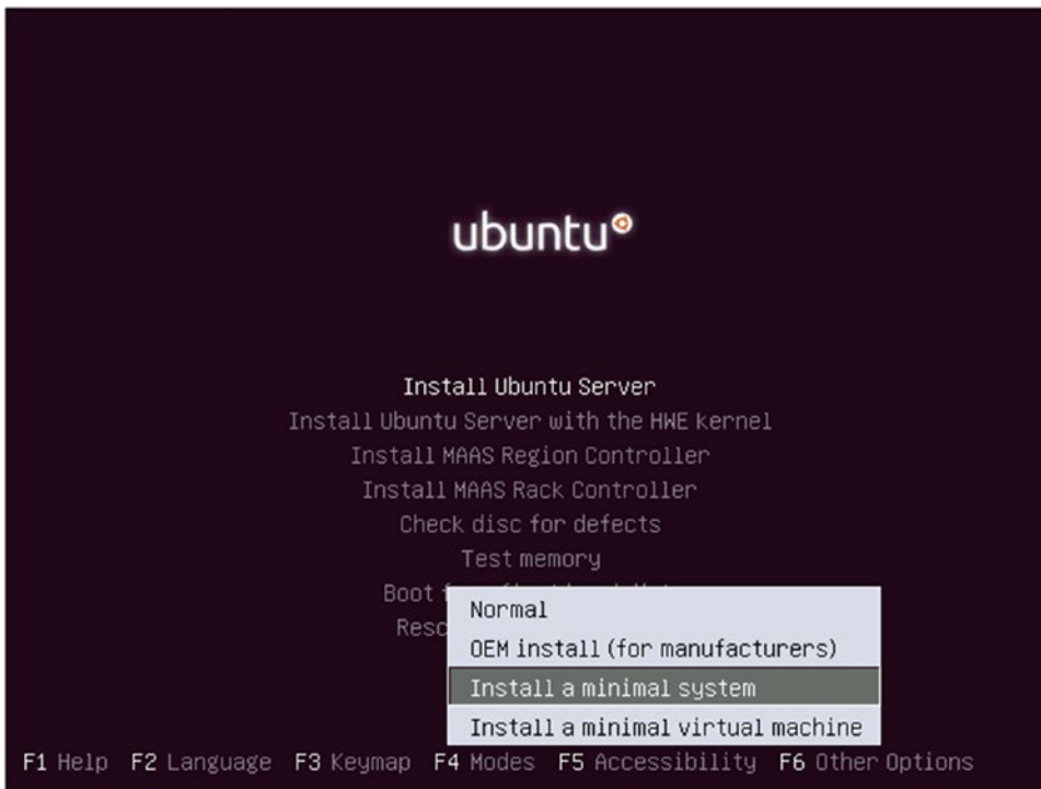
Figure 1-32. Selecting a special install mode is the only difference from an Ubuntu Server install
