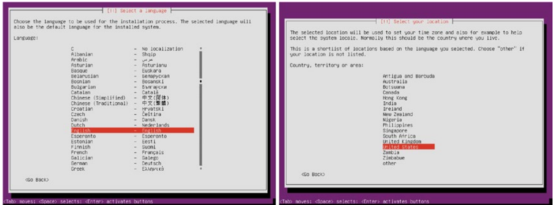
Figure 1-28. The language and locale settings are quite similar to the Ubuntu desktop installer
