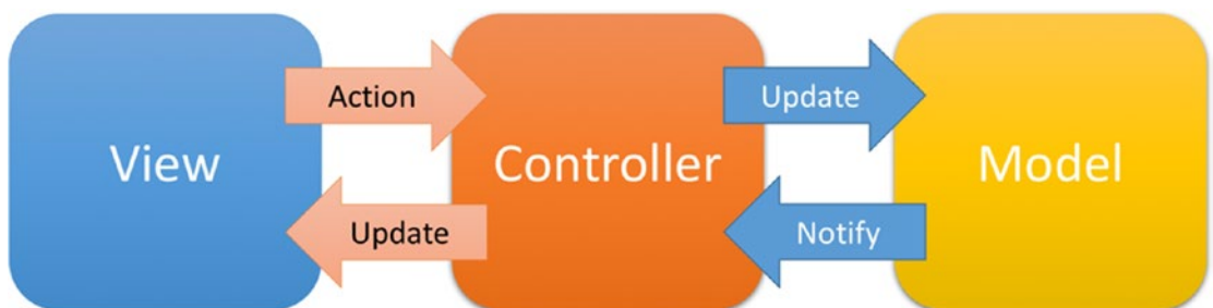
Figure 2-10. A general scheme of the Model View Controller programming paradigm
