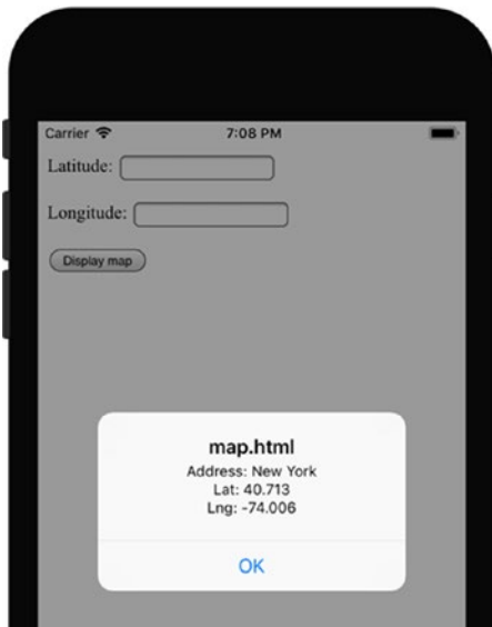
Figure 3-9. Displaying an alert with a JavaScript function invoked through the Web View
