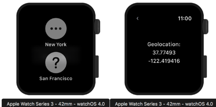
Figure 8-12. Force touch gesture activates the menu, containing a list of cities. When you tap the item, another view is displayed. This view displays the geocoordinates of selected city.
