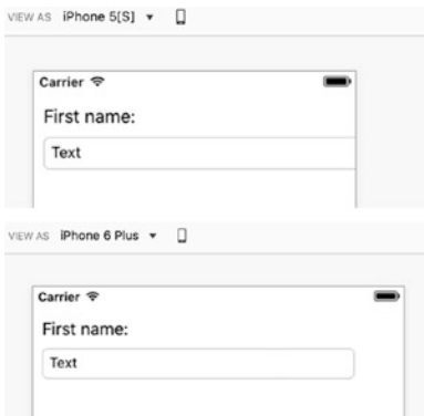
Figure 3-15. Preview of the AutoLayout app on the iPhone 5S and iPhone 6 Plus reveals layout issues
