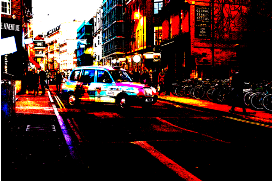
Figure 3-6. Image converted to two values in individual RGB channels
