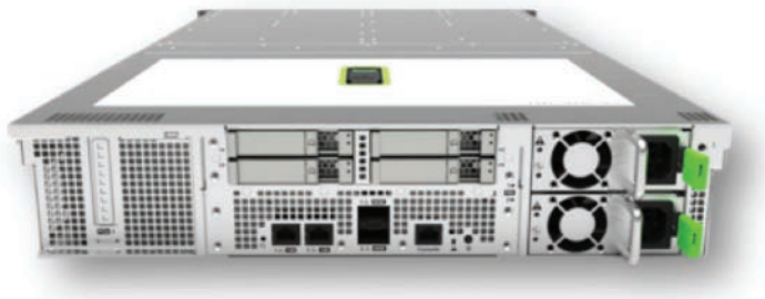
Figure 7-17 Cisco UCS M4308 Modular Server Chassis Front and Rear View
