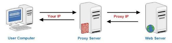
Figure 4-30. How a proxy server works (source: www.darknessgate.com)
