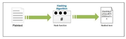
Figure 5-3. How a hash function works
