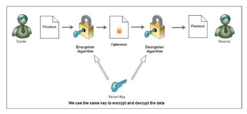
Figure 5-1. Symmetric key cryptography system
