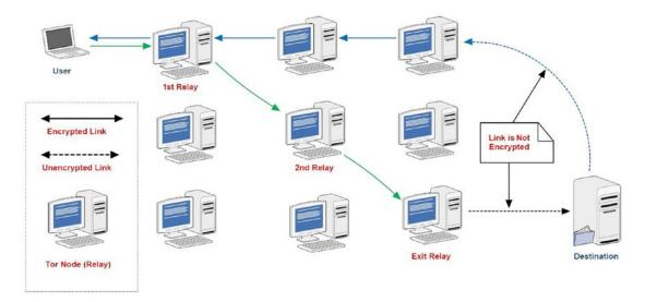
Figure 4-1. How the Tor network works
