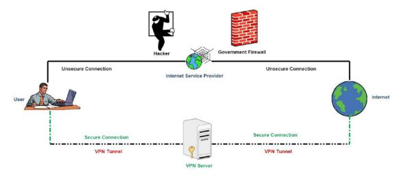
Figure 4-27. How a VPN works (source. www.darknessgate.com)
