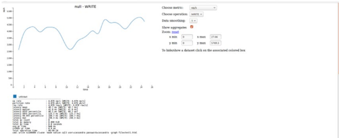
Figure 11-2. A graph of a cassandra-stress tool stress test, generated with the -graph option
