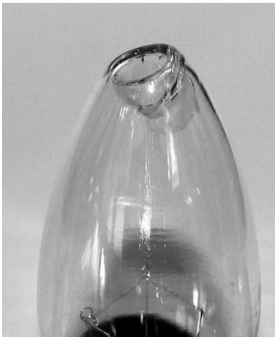
Figure 9-13. The hole in the glass bulb
