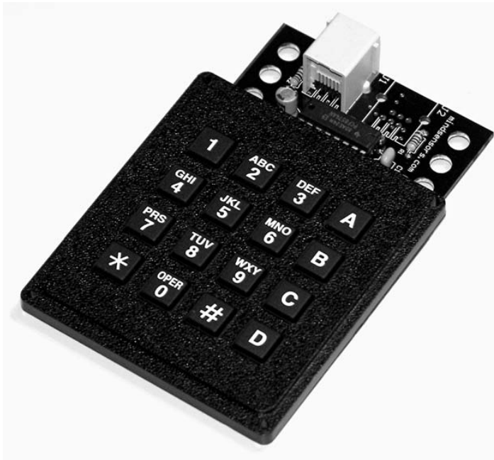
Figure 13-15. Keypad Input built with the Mindsensors Prototype Board
