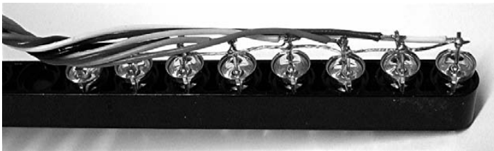
Figure 13-9. Close-up of wand construction
