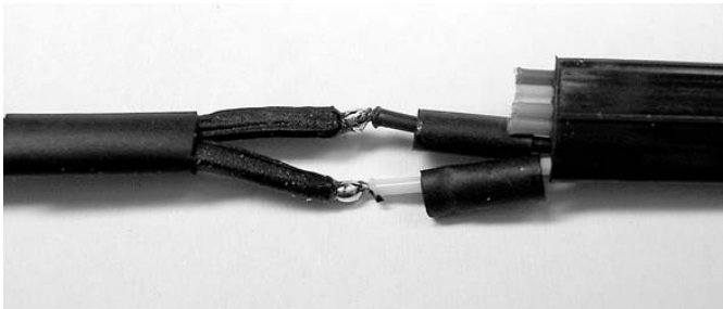
Figure 11-24. Solder RCX and NXT wires together. Don't forget to insert heat shrink tubing!
