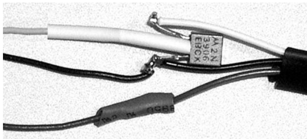
Figure 8-18. Transistor buffer for the GP2D12 interface
