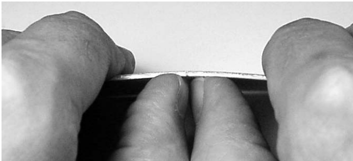
Figure A-9. Snapping the PC board
