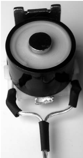
Figure 12-13. Electromagnet coil from 6V relay
