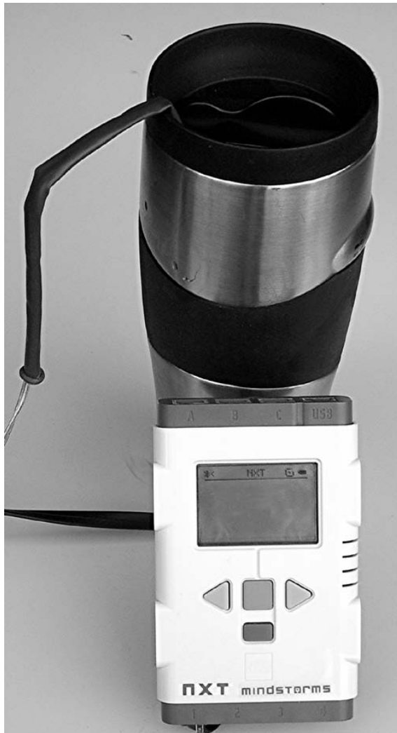
Figure 5-23. Measuring the temperature of ice water
