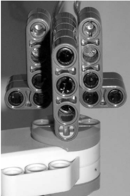
Figure 8-26. Close-up of differential Light Sensor and gnomon
