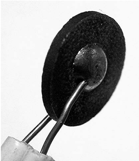
Figure 5-13. Semiconducting pellet inside a thermistor
