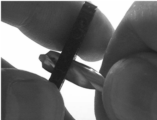
Figure 6-9. Hand drilling triangle beam
