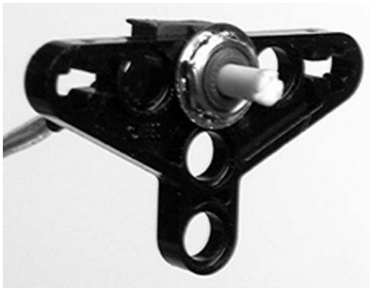
Figure 6-10. Mounted angle sensor
