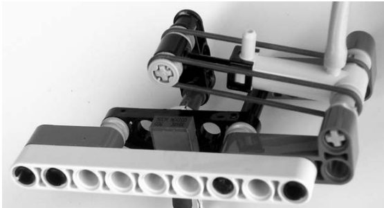
Figure 6-14. Pressure sensor using pneumatic cylinder and 50k \Omega pot
