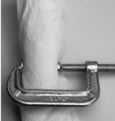
Figure 9-14. Break the bulb with a C-clamp
