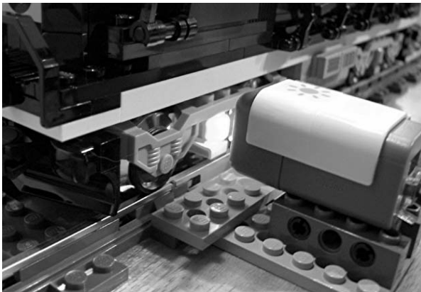
Figure 14-18. Light Sensor as a train detector
