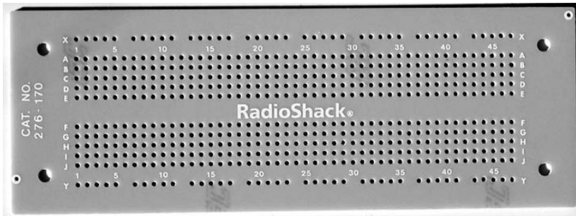
Figure A-6. Printed circuit board that matches the solderless breadboard
