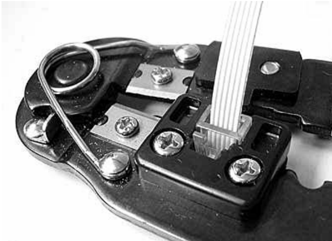
Figure 3-10. Modified RJ-12 crimping tool
