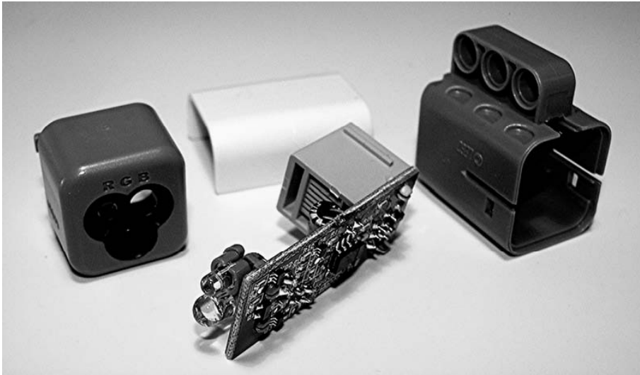
Figure 1-19. Color Sensor breakdown
