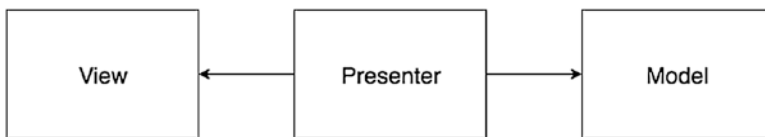
Figure 2-4. MVP diagram where the view is unaware of the model's existence
