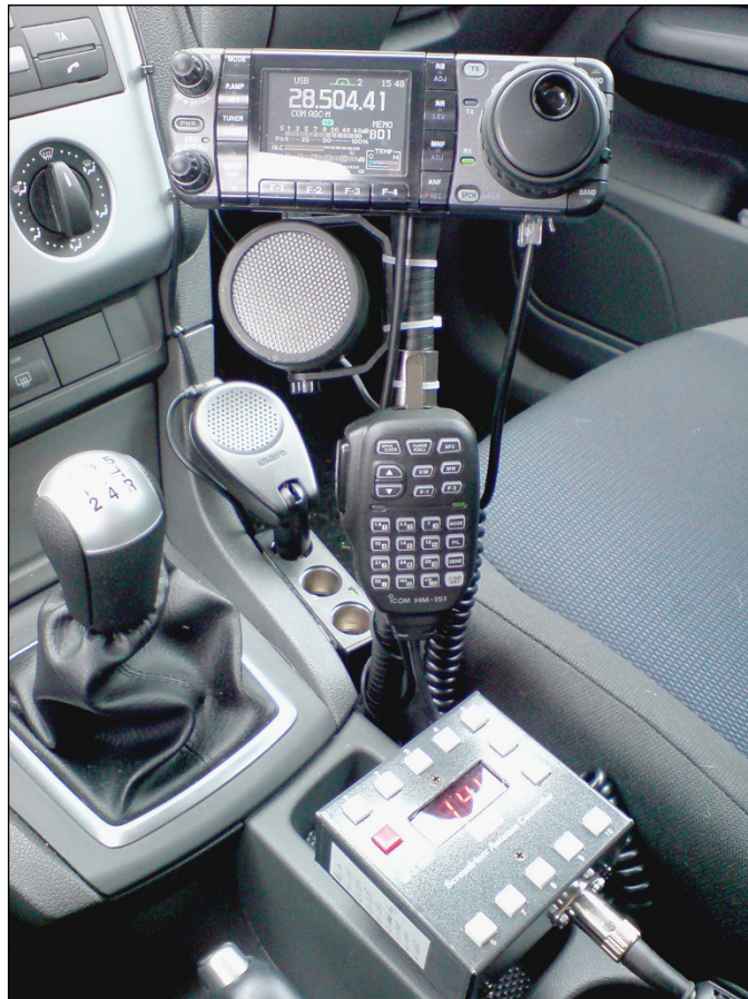
FIGURE 14-4: Most mobile radios have detachable lightweight control heads that are easy to secure on flexible or dashboard mounts.
