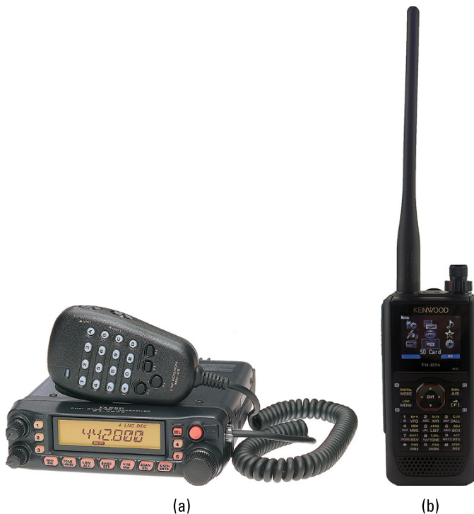
FIGURE 12-1: FM radios: (a) A Yaesu FT-7900A mobile and (b) a Kenwood TH-D74A handheld.
