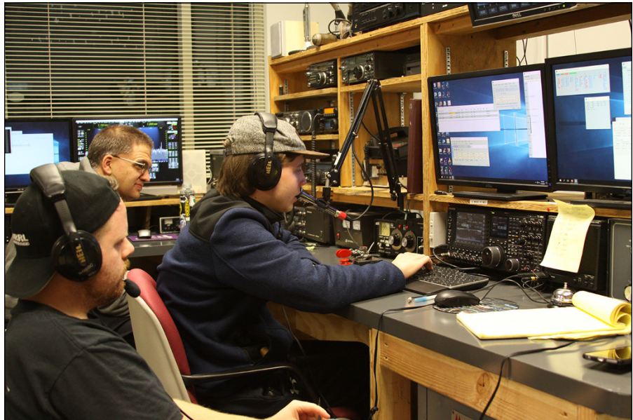
FIGURE 13-4: This multiple-operating-position station organizes gear by function to allow more than one club member to operate at a time.
