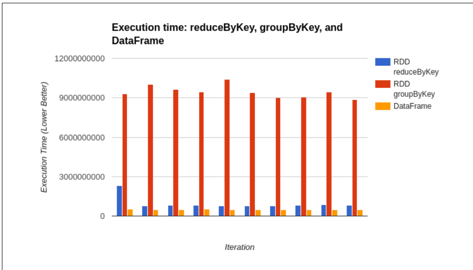
Figure 3-1. Relative performance for RDD versus DataFrames based on SimplePerfTest computing aggregate average fuzziness of pandas
