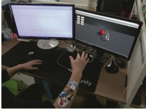
Fig. 2. Based on leap motion system and Ergo LAB, visual feedback - cognitive experiment
