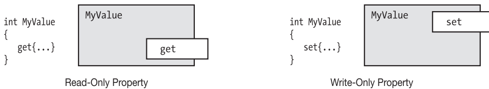
Figure 7-10. A property can have one or the other of its accessors undefined
