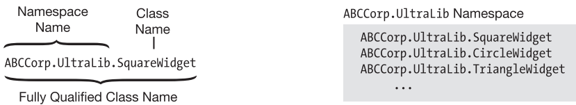
Figure 22-6. A namespace is the set of type definitions that share the same namespace name
