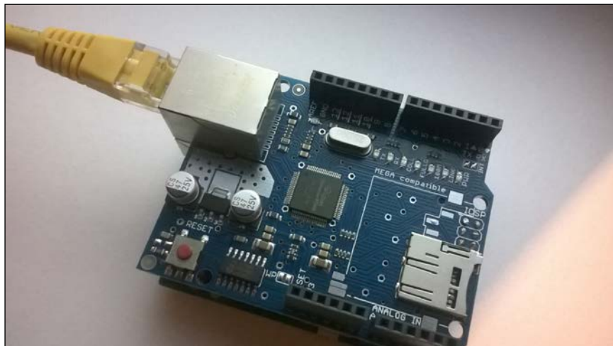
One end of the Ethernet cable is connected to the Arduino Ethernet board
