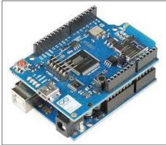
Arduino WiFi Shield is stacked with Arduino UNO
