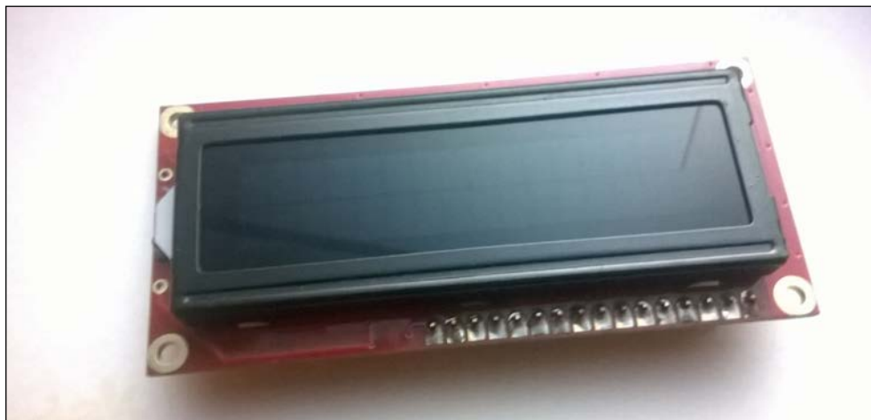
Hitachi HD44780 driver compatible LCD screen (16 × 2) – Top View
