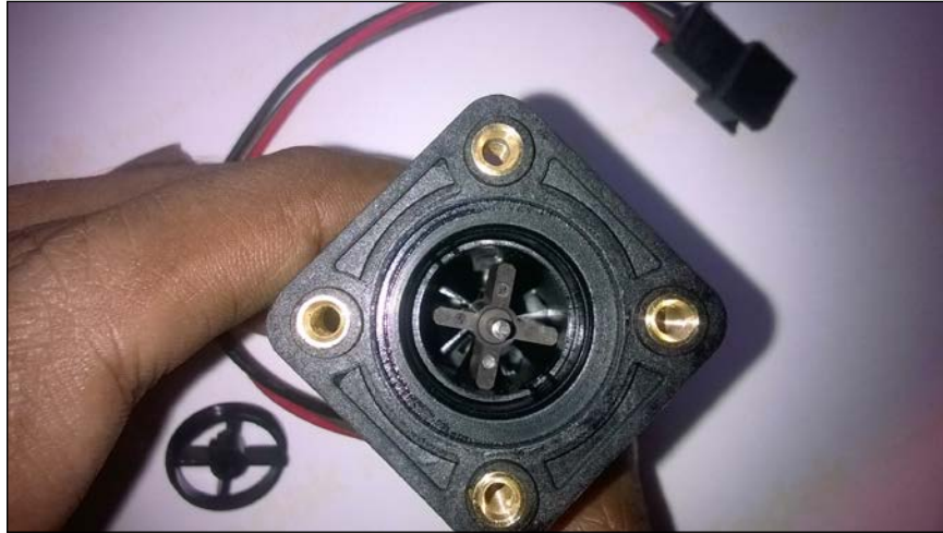
Pinwheel attached inside the water flow sensor
