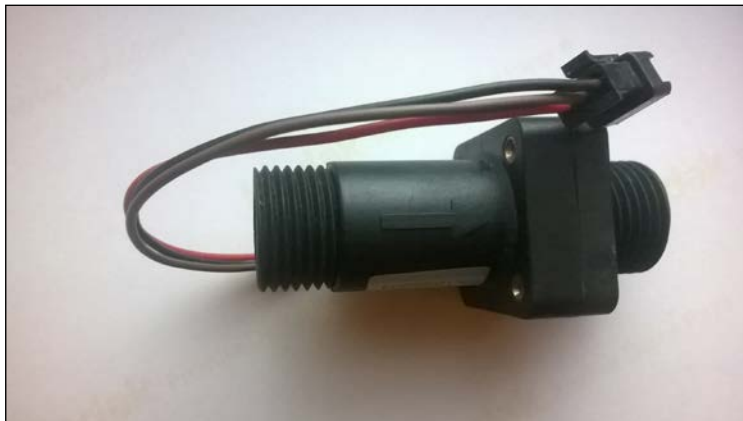
Liquid flow sensor - the flow direction is marked with an arrow
