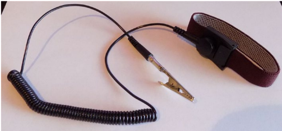
Figure 1-1. A strap used to ensure static electricity cannot damage evidence. Copyright (c) 2017, PeteFinnigan.com Limited. Used with permission.
