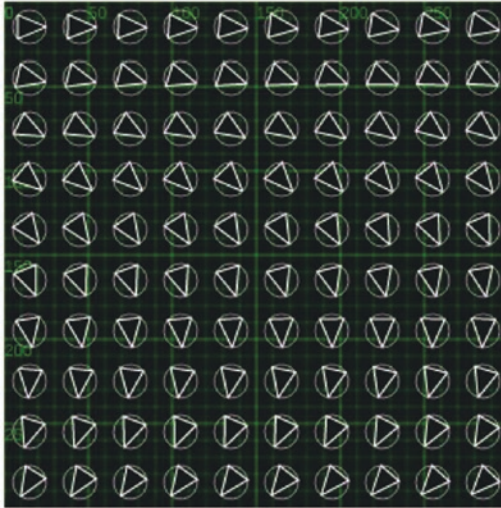
Figure 4-6. Controlled ship drawing using canvas transformations
