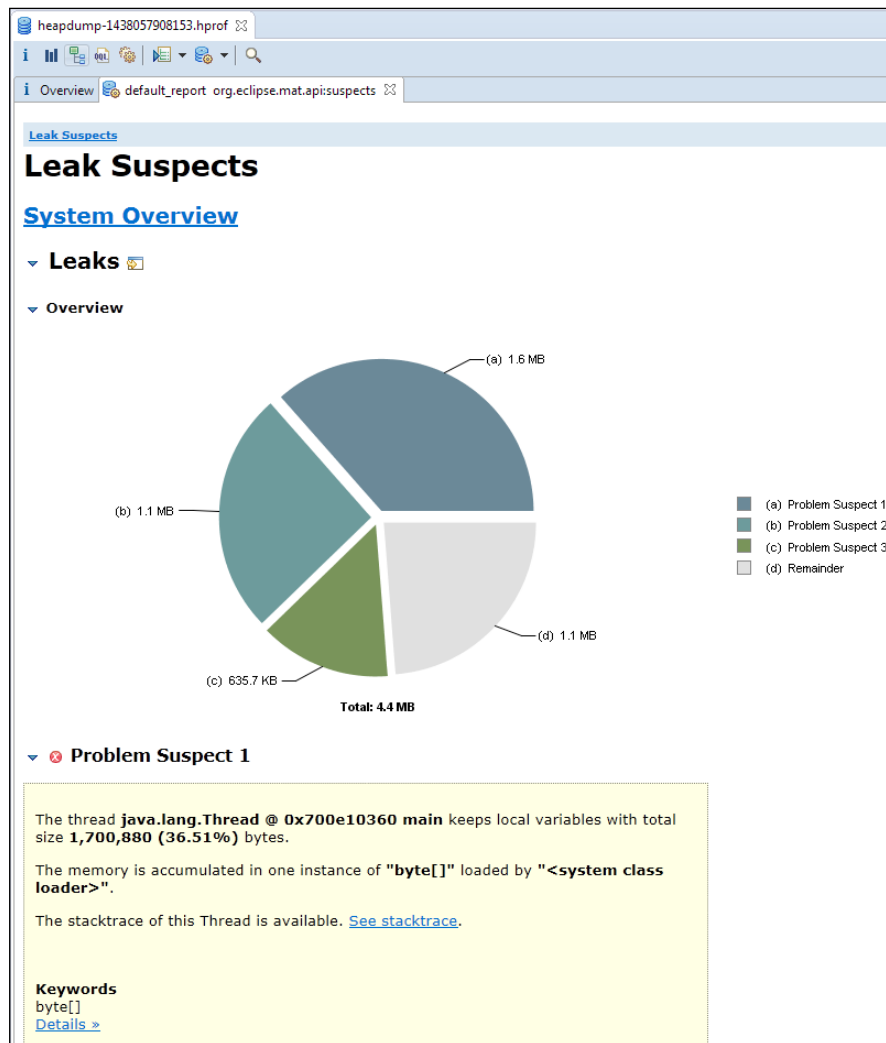
Figure 11.13 Eclipse Memory Analyzer: Leak Suspect report
