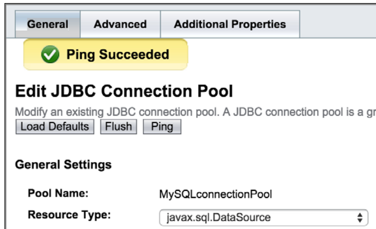
Figure 7.11 Test JDBC Connection Pool in GlassFish
