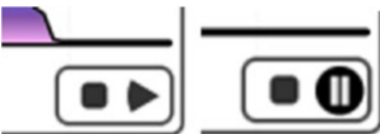
Figure 9-2. Custom button panel control with Stop (rectangle), Play (triangle), and Pause (circle) buttons
