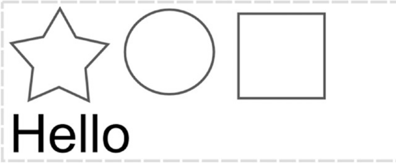
Figure 5-5. A FlowPane layout with nodes flowing left to right with the ability to wrap nodes based on horizontal space. The Hello text node is wrapped to the next line because the available horizontal space, denoted by the dashed line, is too small.
