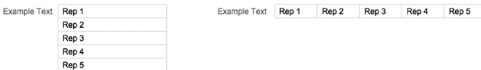
Figure 30-29. A text field defined with five repetitions displayed on a layout in both vertical and horizontal arrangement
