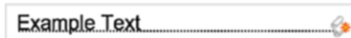
Figure 37-4. The object badge visible on a field with one or more script triggers assigned
