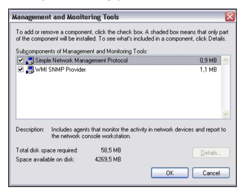
Then select both SNMP and WMI SNMP Provider from the next window to proceed with the installation of SNMP management and monitoring tools:
