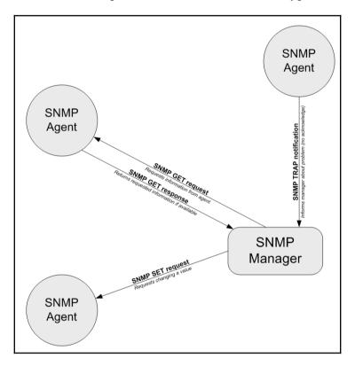
SNMP has several versions that an agent can communicate over. **SNMPv1** was the first version of the protocol. This featured get, set, and trap operations. The standard defined scalar data objects as well as tabular objects. It also featured the getnext operation, which allows iterating over the tables of data objects.
