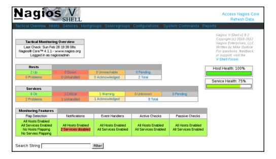
The V-Shell interface is very similar to the Nagios web interface; the main differences are that it does not use frames and the menu is shown on the top rather than on the left. The menu is also a drop-down menu, and hovering over one of the menu items shows a list of available elements.
