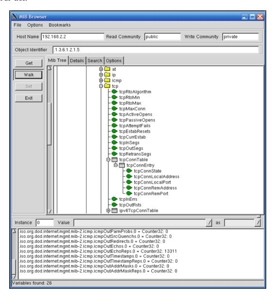
Another interesting tool is **Tcl/tK based Interactive Network Editor** (**TkIned**) from the Scotty package (https://sourceforge.net/projects/tkined-scotty/). This is a graphical tool that uses Tk for the graphical interface and Scotty for the SNMP protocol. It allows browsing of the MIB tree, the monitoring of hosts over SNMP, and the visualization of your network by clicking on the layout.
