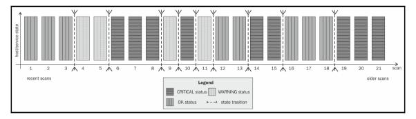
Nagios then finds all of the changes between different states and uses them to determine if a host or service state is flapping. It checks to see if a state is the same as the result from the previous check, and if it has changed, a state transition is counted at this place. In the preceding example, we have nine transitions.
