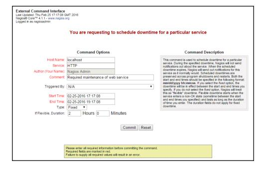
The form consists of the host and service name, a comment, and an optional option list to choose a downtime that triggered this host/service to also be down. When specifying time during which the downtime should be scheduled, it is possible to enter **Start Time** and **End Time** or use the **Duration** field. If you want to specify how long the offline will take, choose **Flexible** in the **Type** field. Otherwise choose **Fixed** to specify the start and end time.
