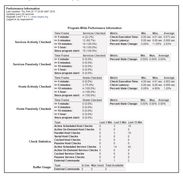
The page contains information on the number of host and service checks performed within various periods of time as well as the number of reports received from external applications. It also contains a number of commands received from external applications; this usually means the web interface.
