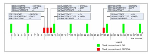
Event handlers are triggered for each state change—for example, in minutes, 10, 23, 28, and 29. When writing an event handler, it is necessary to check whether an event handler should perform an action at that particular time or not. See the preceding example for more details.
