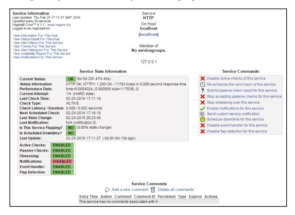
The main table on the left shows detailed information on the service, namely the current status, output from the check, and detailed information on the last and next planned checks. The page also shows whether the service is flapping along with the flapping threshold and when the last notification was sent out.
