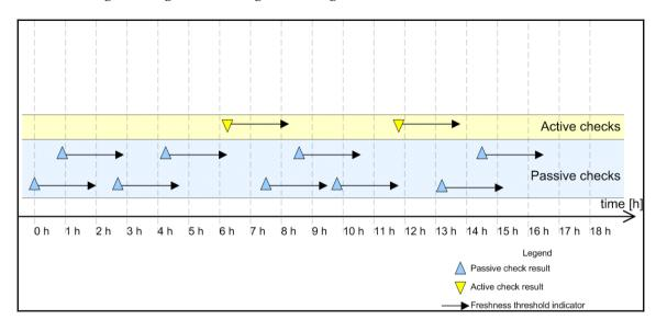
The following is a diagram showing when Nagios will invoke active checks:
