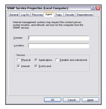
The window has three additional tabs—**Agent**, **Traps**, and **Security**. The **Agent** tab allows you to configure which parts are exported over SNMP, and offers the setting up of contact and location information.
