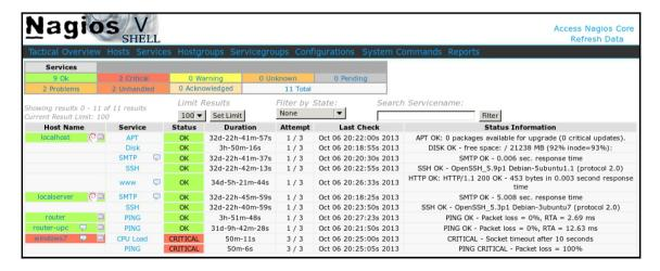
Nagios V-Shell provides views for most of the options available in the standard web interface. It also uses JavaScript for many operations, which makes it faster than the standard web interface. This is especially important for mobile devices that often have slower network connectivity.
