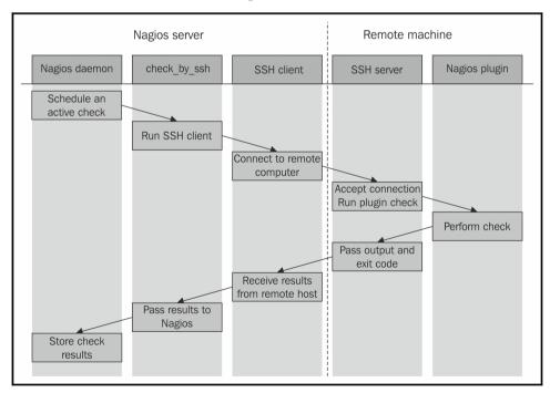
Once Nagios schedules an active check to be performed, the <code>check\_by\_ssh</code> plugin runs the <code>ssh</code> command to connect to the remote host's SSH server. It then runs the actual plugin, which has to be present on the remote host, and waits for the result. The SSH client passes the standard output as well as exit code to the <code>check\_by\_ssh</code> plugin that also prints the output and exits with the same code as the plugin.
