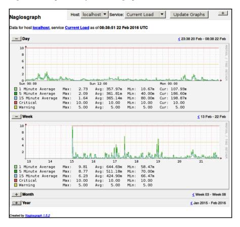
Graphs support zooming in and out using the mouse. To zoom in, simply select a range to zoom in using the left mouse button. The graph will zoom in to that data. To zoom out, simply click the right mouse button.
