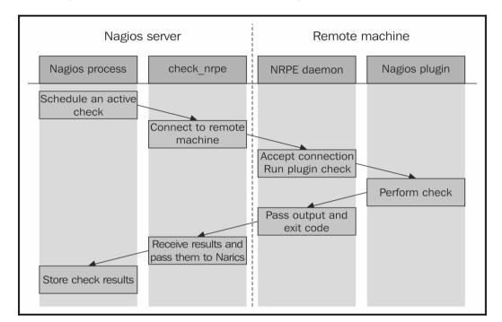
The following is an illustration of how such a check is performed:
