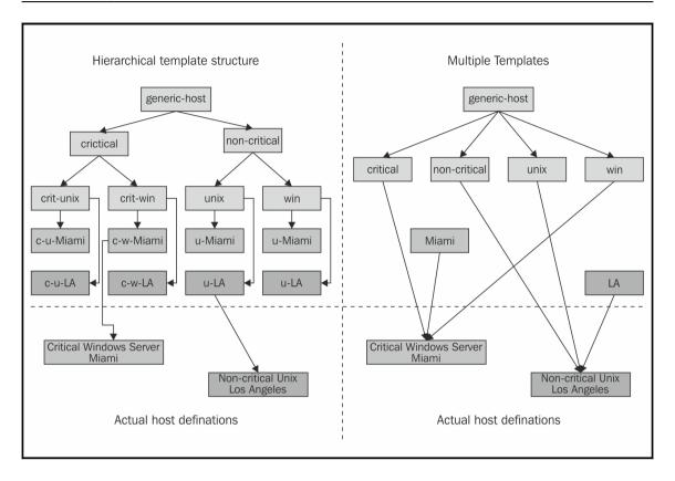
This example illustrates how the templates can be structured using both hierarchy and multiple templates inheritance. It shows how to use templates for host definitions, but similar rules apply for services as well; the inheritance structure may be a lot different, though.
