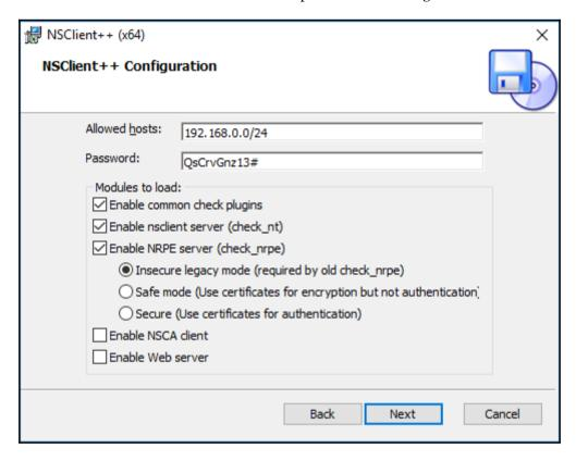
The **Allowed hosts** should be set to the IP address and/or IP address ranges of machines that will be performing the checks, such as 192.168.0.0/24, if that is the IP address range of your local network.
