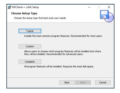
If unsure, it is recommended that you perform a complete installation, but advanced users may wish to choose which features to install. The installer will also ask for the location to install itself. Unless you need to install NSClient++ in a specific location, it is best to use the default path of C:\Program Files\NSClient++.
