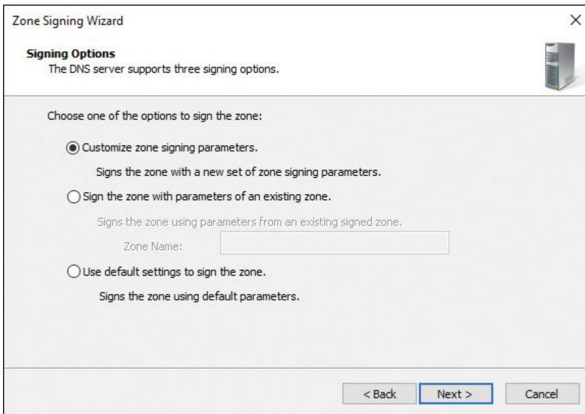
Figure 4-4 Signing Options Page of the DNSSEC Zone Signing Wizard on a Windows Server 2016 DNS Server
