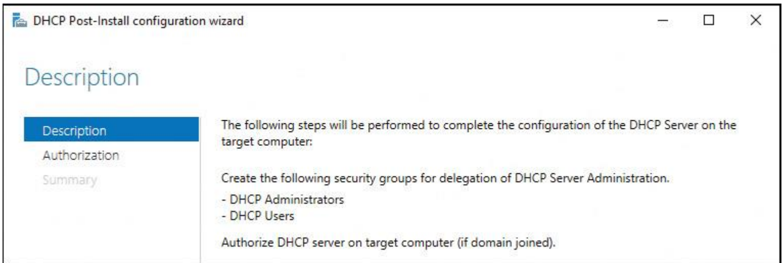
Figure 6-5 DHCP Server Post-Install Configuration Wizard (Description)
