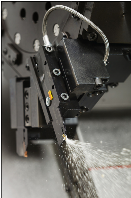
FIGURE 12-3: Always use coolant through the tool inserts, drills, and toolholders whenever possible, preferably with high-pressure coolant.
