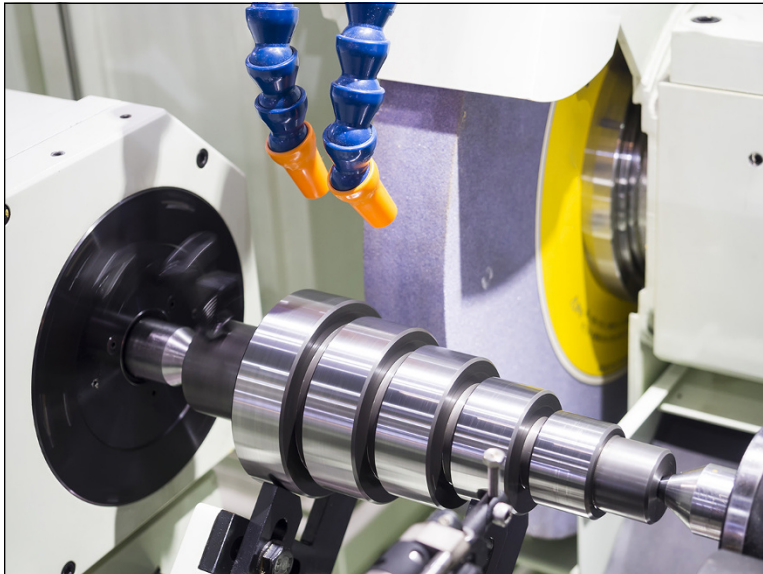
FIGURE 3-3: Cylindrical grinding is one of most accurate of all machining processes.
