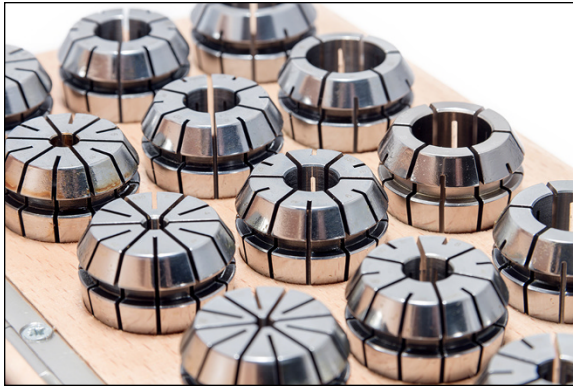
FIGURE 7-2: The four-decades-old ER collet is one of the most commonly used toolholding systems.
