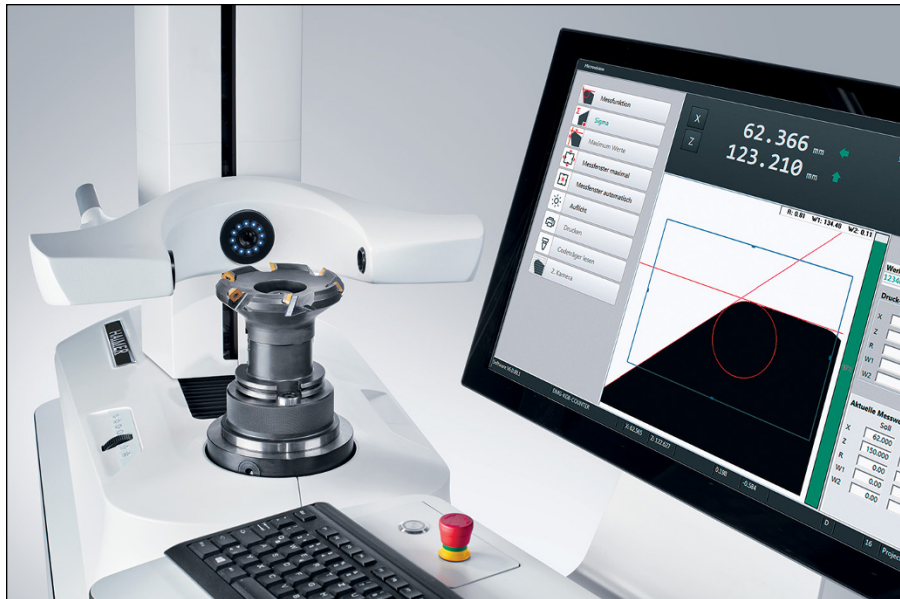
FIGURE 8-5: Offline tool presetting is one of the best ways to decrease downtime and reduce the risk of machine crashes.
