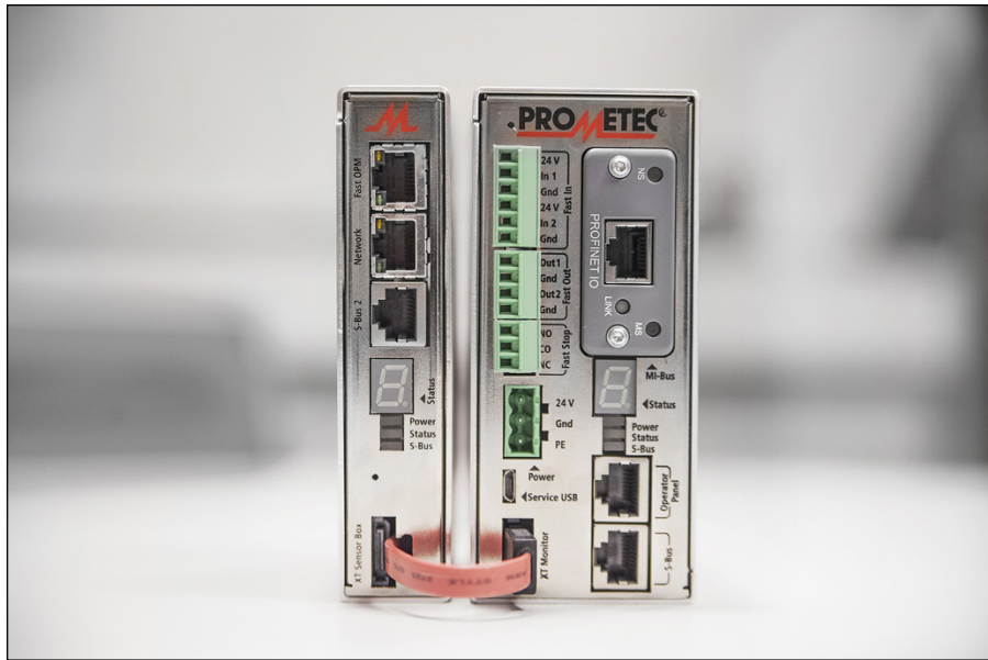
FIGURE 13-3: Machine-tool monitoring devices assure process safety by detecting tool wear, broken tools, and collisions, and stopping the machine before further damage can occur.
