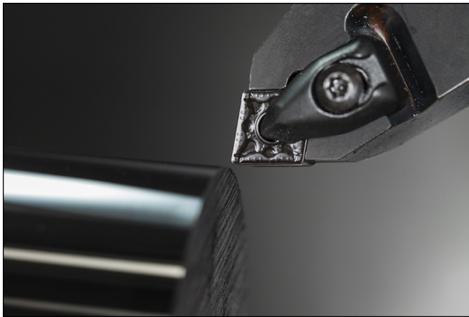
FIGURE 7-6: An 80-degree diamond indexable turning tool. Like all precision tooling, stick tools should be given a little TLC for the best machining results.
