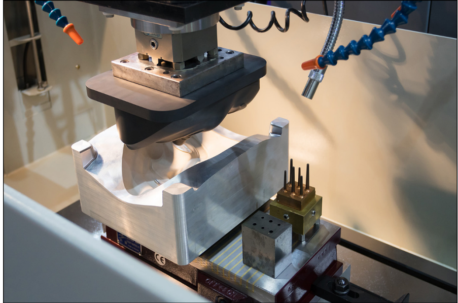
FIGURE 3-1: A graphite EDM electrode is used to machine an aluminum mold cavity.
