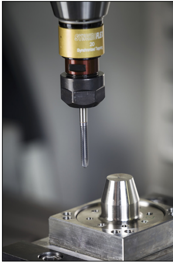
FIGURE 5-2: Tapping is one of the most common threading operations.
