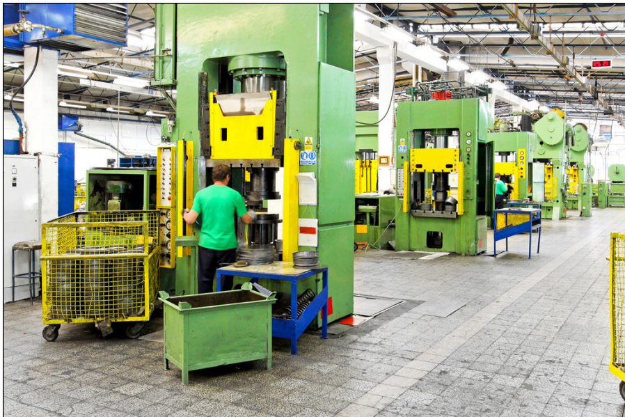
FIGURE 3-7: Stamping machines like these are used to trim and form parts.
