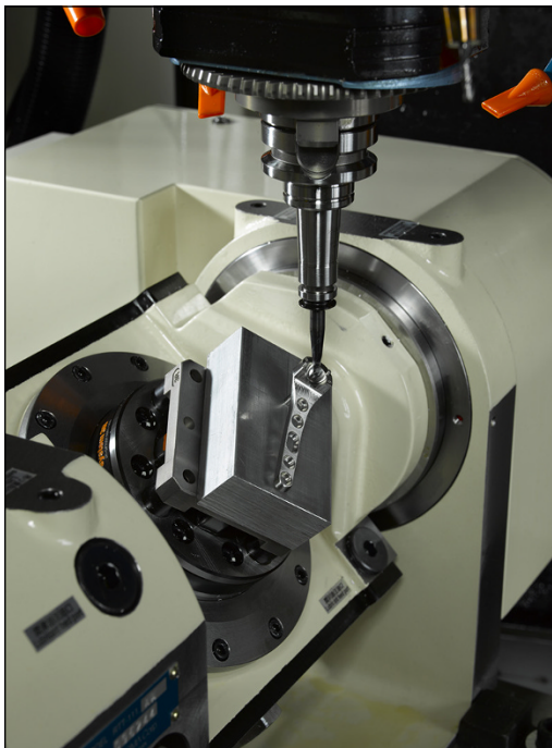
FIGURE 2-4: A trunnion table is the next best thing to a five-axis machining center. Note the A and B axes “rotary on a rotary” table design.
