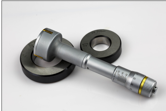
FIGURE 10-3: Of all the different kinds of inside micrometer, the tri-mic shown in this picture is the most flexible and easy to use.
