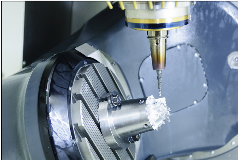
FIGURE 6-5: Five-axis machining centers need vises and fixtures that provide plenty of clearance.
