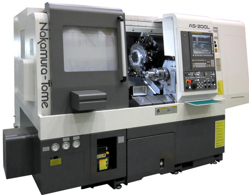
FIGURE 2-5: This two-axis lathe has a sub-spindle instead of a tailstock, allowing both ends of the part to be machined in a single setup.
