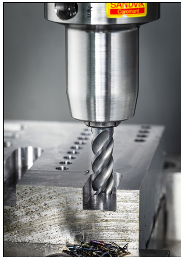
FIGURE 5-3: A four-flute carbide end mill cutting a slot in a piece of carbon steel.
