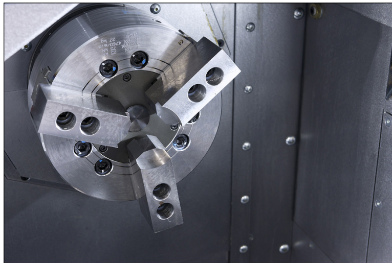
FIGURE 6-1: A three-jaw chuck mounted on a CNC lathe. The “soft” jaws on top have been machined to hold a piece of round material.
