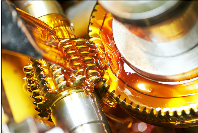
FIGURE 3-5: Hobbing is an important process for high-production gear manufacturing.
