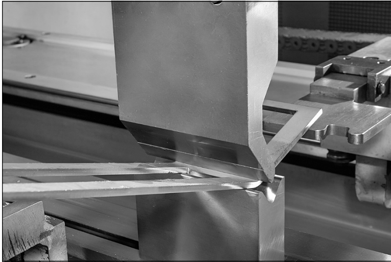
FIGURE 3-6: Press brakes produce complex bends in sheet metal.
