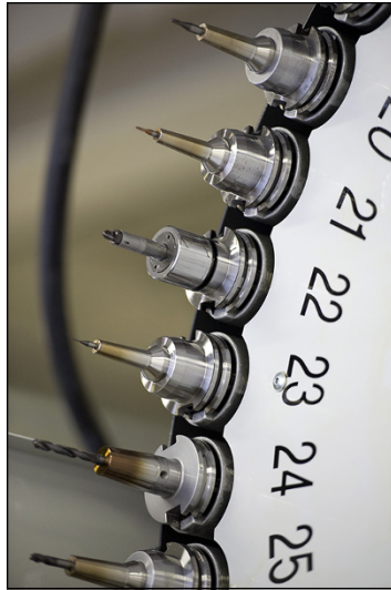
FIGURE 7-4: An assortment of CAT40 toolholders in a machining center carousel. Note the thermally discolored ends, identifying them as shrink fit holders.
