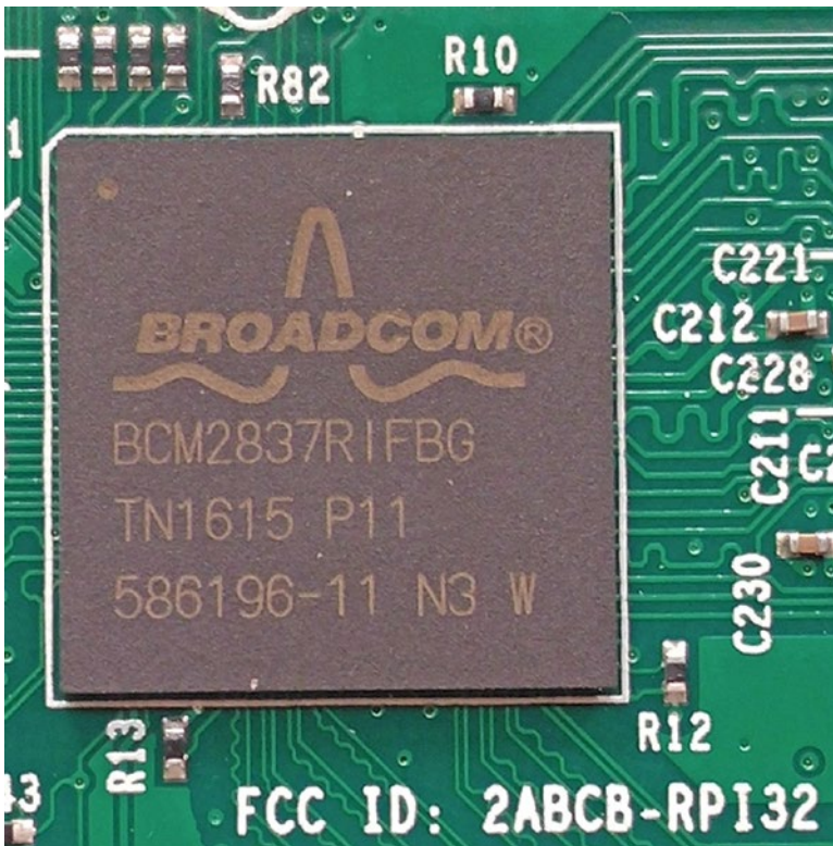
Figure 1-4. The Broadcom System on a Chip is the heart of the Raspberry Pi
