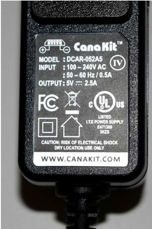
Figure 2-3. Volatage and current ratings are on adapters as shown here
