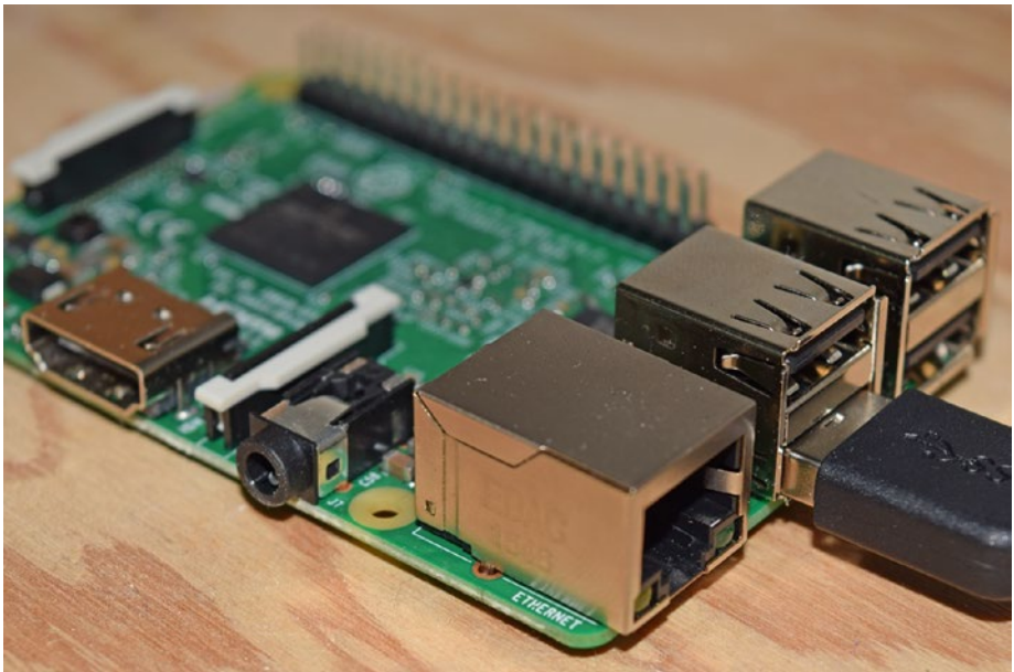
Figure 7-5. A Raspberry Pi 3 with the 3.5mm jack at the edge of the board center. To the left is the HDMI jack, and on the right edge are four USB receptacles with a cable plugged into one.
