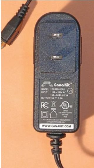
Figure 2-5. This power supply was included with my most recent purchase of a Raspberry Pi 3 and is designed specifically for that board
