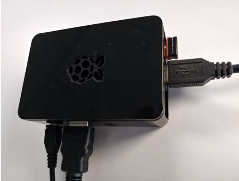
Figure 4-2. Raspberry Pi 3 configured and connected as a media center controller
