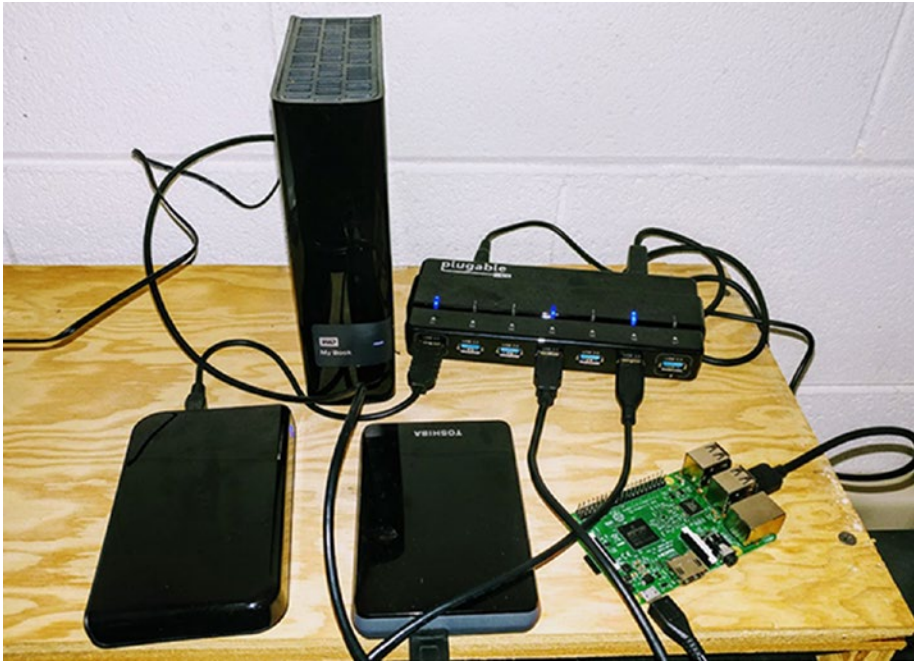
Figure 3-9. My Raspberry Pi Model 3 with 5TB of drives and a powered USB hub
