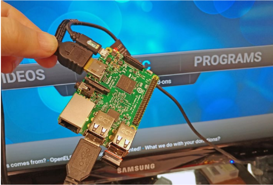
Figure 5-1. The Raspberry Pi 3 has the memory and processing power needed for running your home theater
