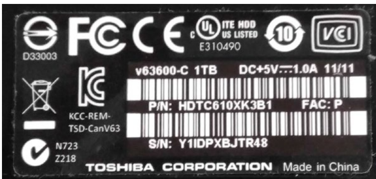
Figure 2-6. This 1TB portable hard drive requires 1.0 A as shown on its label
