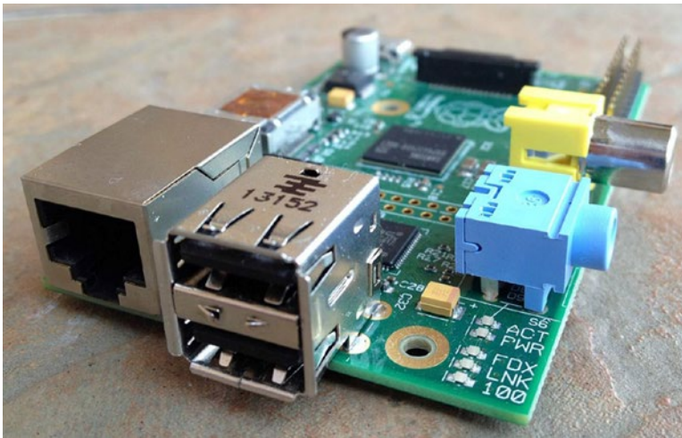
Figure 1-2. The Model B had a network port and two USB receptacles. Newer models provide four USB receptacles. (Photo Justin Goetz, Creative Commons).
