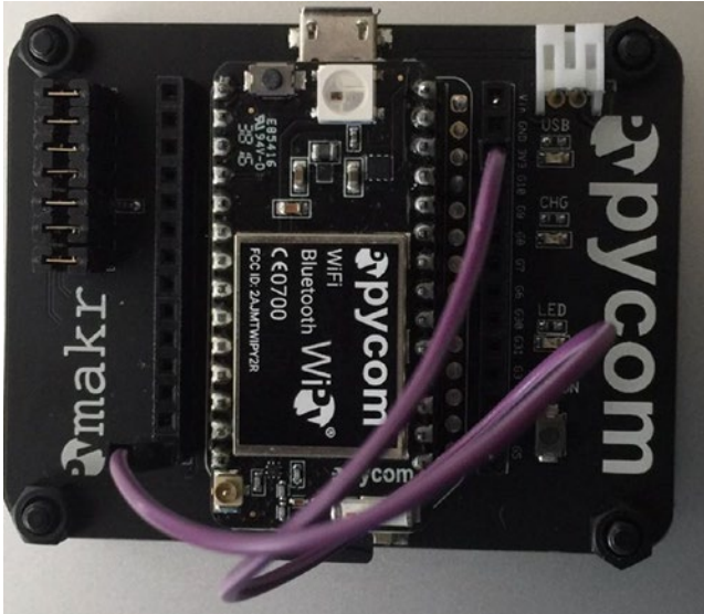
Figure 3-16. Jumper Installed for Safe Boot Selection (WiPy Expansion Board)
