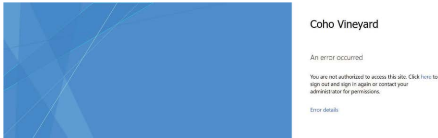
Figure 3-40 AD FS WAP sign-in page showing access blocked by a claims rule
