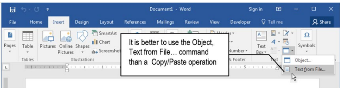
Figure 11-33. Use the Insert ► Object ► Text from file tool to select all the text of another Microsoft Word document and inserting at the current cursor position
