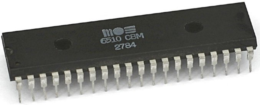
Figure 9-2. The CPU of a primordial Commodore 64 computer. Photographed by Konstantin Lanzet.
