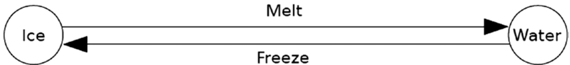
Figure 22-2. State diagram applied to ice changing state to water and water changing state to ice
