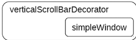
Figure 16-6. simpleWindow wrapped by verticalScrollBarDecorator
