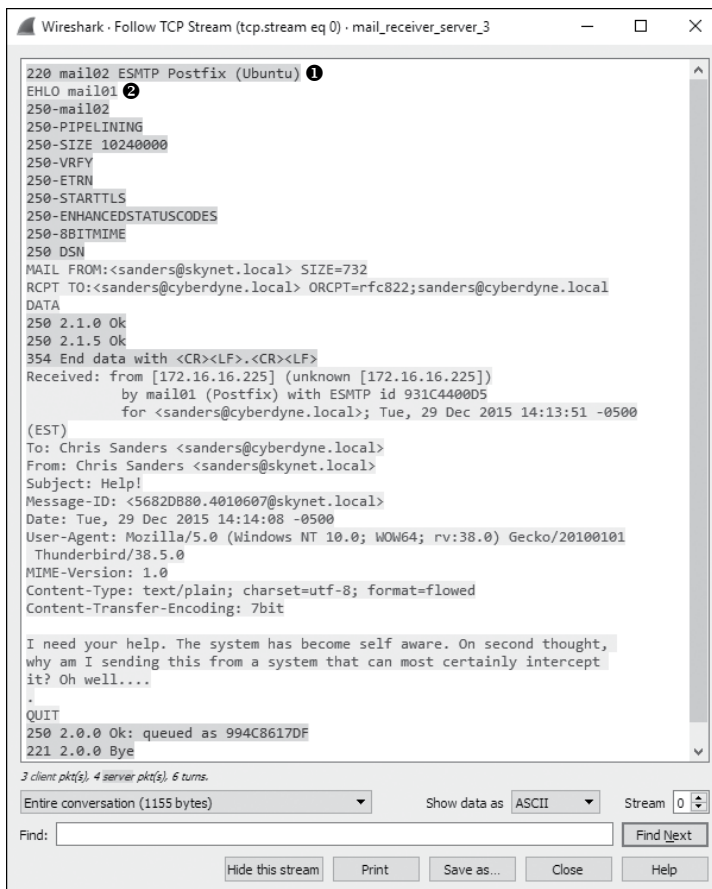
Figure 9-32: Viewing the TCP stream from the local email server to the remote email server
