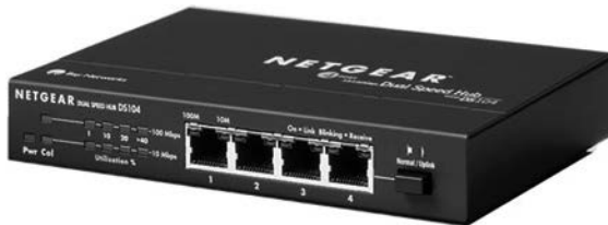
Figure 1-4: A typical 4-port Ethernet hub
