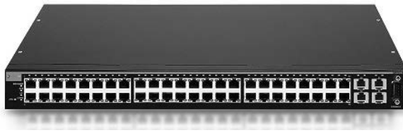
Figure 1-6: A rack-mountable 48-port Ethernet switch
