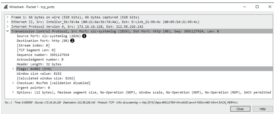
Figure 8-3: The source and destination ports can be found in the TCP header.
