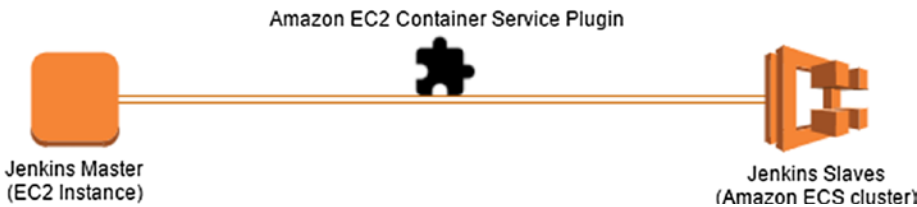
Figure 4-10. Scalable Jenkins Slave cluster using ECS Instances
