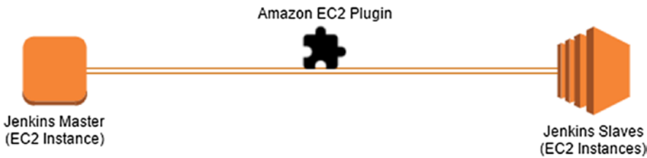
Figure 4-9. Scalable Jenkins Slave cluster using EC2 Instances
